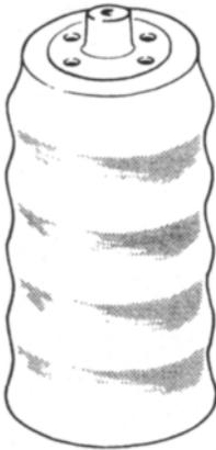
**Fig. 6.7** Nominal 6 V sealed nickel–cadmium battery formed by connecting five cells in series. (By courtesy of Varta.)
