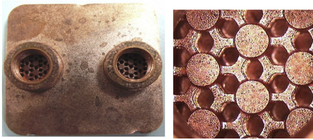
Figure 6.1.15 Images of a honeycomb heat sink and its microstructure, with a unit cell represented in dashed line.
