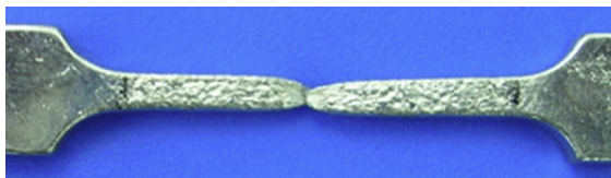
Figure 6.2.2 Typical ductile failure mode of solder bar.
