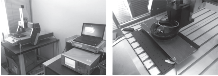
Figure 5.19 (a) Scanned H_y on the surface of a certain microstrip-type differential line without and with the CMF, and (b) and the measurement setup.
