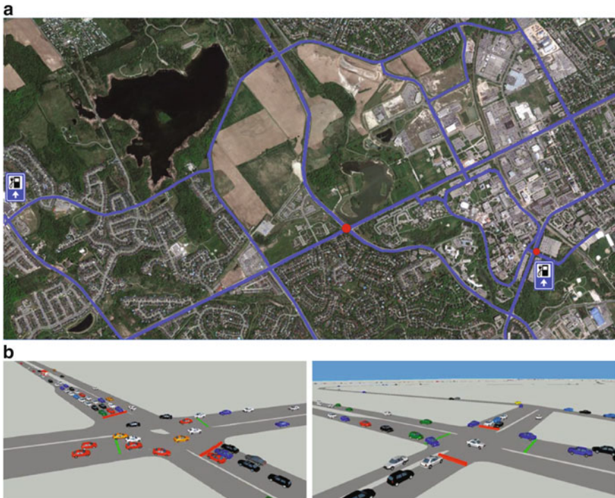
Fig. 3.4 The simulation scenario of University of Waterloo region in VISSIM. (a) A snap shot of the simulation region with signing the simulated roads in blue. (b) The 3D vehicle traffic illustrations of two intersections highlighted in red on the upside
