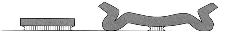
Figure 6.25 A small bump is placed at the bottom of the structure to prevent adhesion
