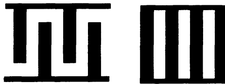
Figure 13.1 Basic elements of a SAW-IDT microsensor: IDT (left), spacing and reflector (right)
