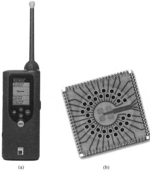
Figure 15.8 (a) A commercial handheld electronic nose from Cyrano Sciences and (b) its 32-element polymer composite (black dots) screen-printed chip. The four central squares are thermistors, and a heater pad has been printed on the reverse side
