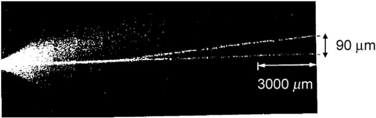
**Figure 10.22** Y-coupler written by fs-laser method. Light entering from left is split in the y-section (taken from Ref. [23]).
