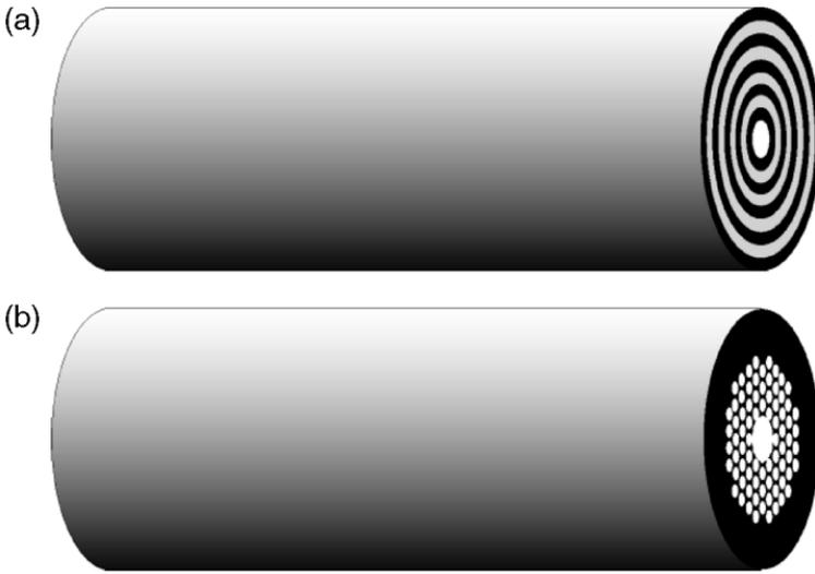
**Figure 9.15** (a) Schematic drawing of a hollow-core Bragg waveguide. (b) Schematic drawing of a hollow-core waveguide in a triangular lattice.
