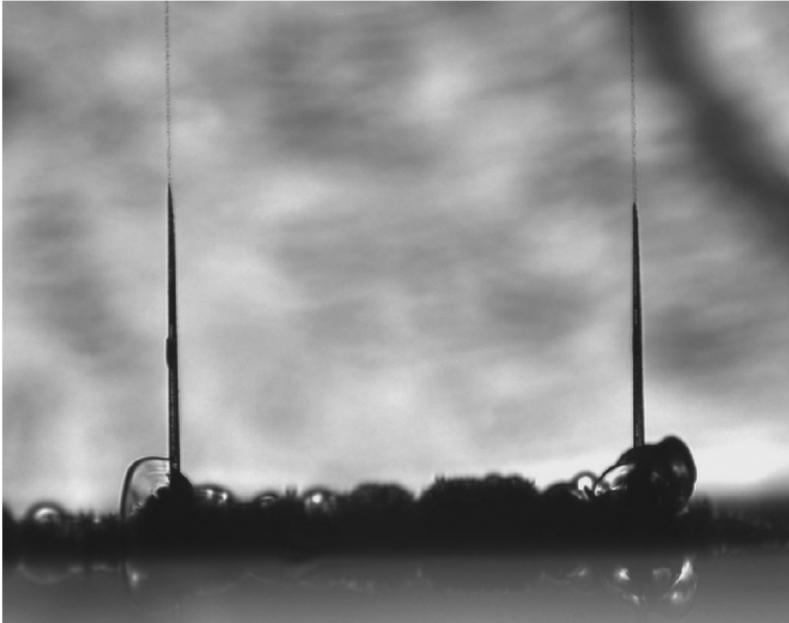
**Figure 10.31** Photomicrograph of fs-laser hole drilling in silica. See text for explanation of the technique.
