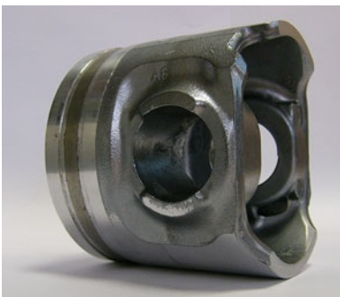
Fig. 1 Image of an aluminium piston with iron ring insert for diesel motors
