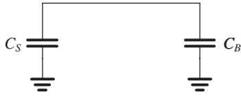
Figure 16.19 When the voltage of the selected word line is raised, the transistor conducts, thus connecting the storage capacitor C_S to the bit-line capacitor C_B .
