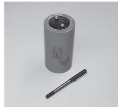
Figure 3.51 (a) Half-wave rectifier circuit with filter capacitor; (b) a-175,000- \mu\text{F} , 15-V filter capacitor. Capacitance tolerance is -10 percent, +75 percent.
