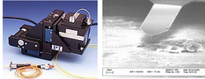
Figure 8.9. Left: configuration of a 6-dof hybrid micromanipulator (magnetic and piezoelectric actuators) and right: AFM cantilever with piezoresistive force sensor
