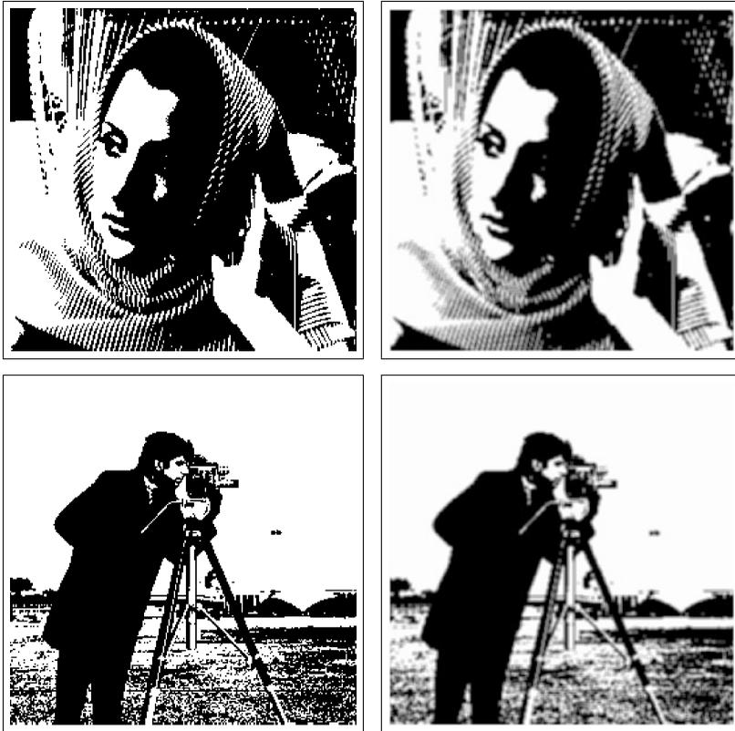
Fig. 29 Inverse half-toning memristor cellular automaton. Initial state binary images (left) are converted into 10-gradations grayscale images (right)
