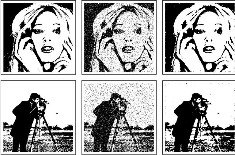
**Fig. 28** A noise removal memristor cellular automaton. Binary images, Gaussian noise images (noise level 2 %), and noise removed images are illustrated from *left to right*
