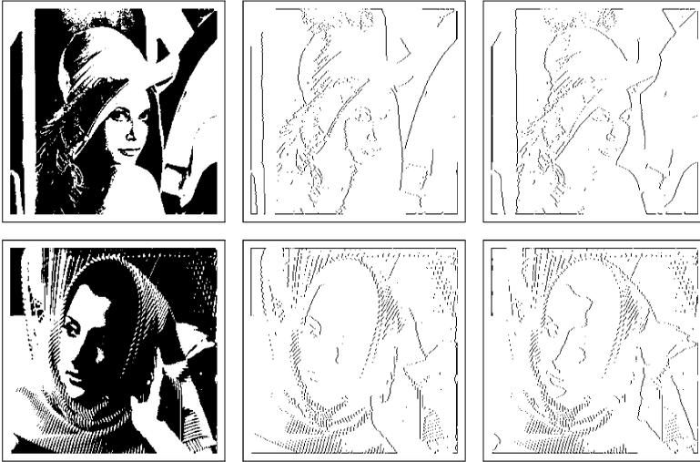
**Fig. 37** Right and left edges detection memristor DTCNN. Right edges and left edges in binary images are detected. Input images, output images of right edge detection, and output images of left edge detection are illustrated from left to right
