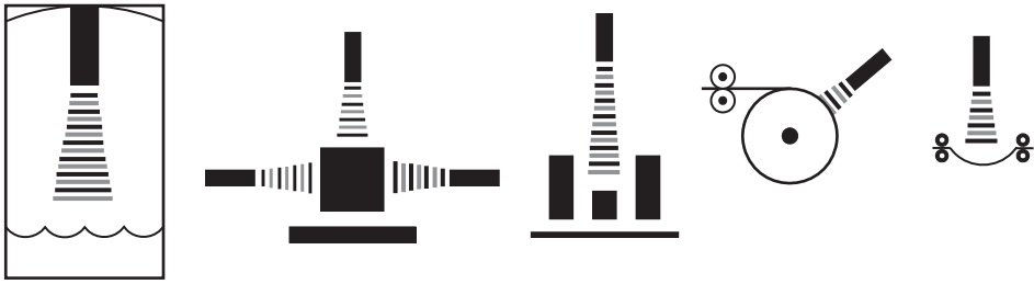
FIGURE 6.28: Applications of of a sonic distance sensor in various manufacturing processes: (a) liquid level sensing, (b) two-dimension sensing (i.e., box height and width), (c) one-dimension sensing (i.e., box height), (d) roll diameter sensing, (e) web slack sensing.
