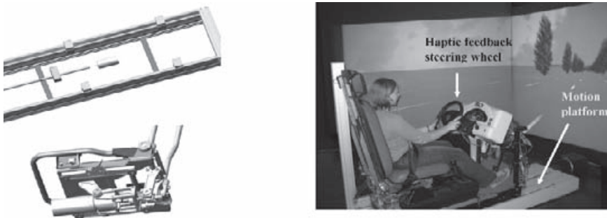
Figure 1: The driving simulator: CAD model of the motion platform and seat (left), overview (right)
