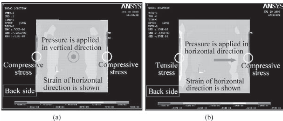
Figure 4: FEM result of distortion of a diaphragm.
