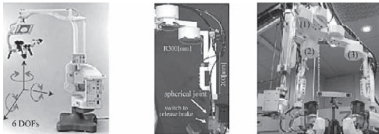
Figure 2: (left) microscope arm, (center) six-DOF precise positioning arm, (right) three arms for each manipulator
