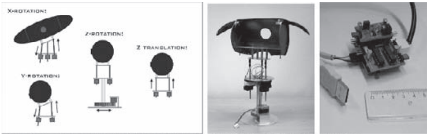
Figure 2, Neck movements (left), Head and Neck unit (center), and Atomi boards (right).
