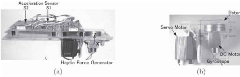
Figure 2: Experimental device for haptic illusion (size: 80 \times 225 \times 88 mm, weight: 0.386 kg). (a) Overall view; (b) Haptic force generator
