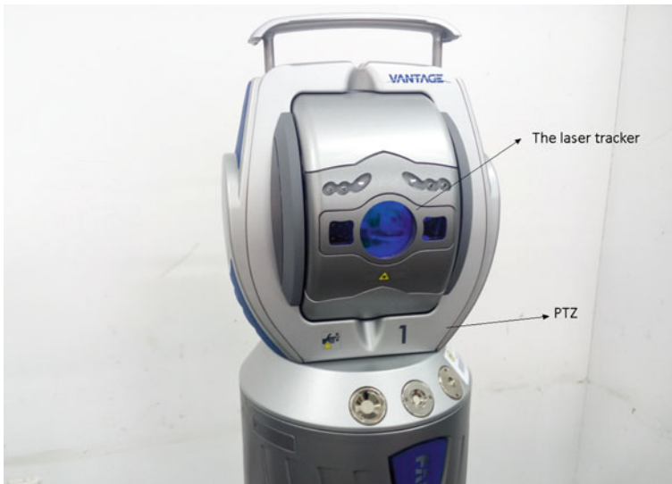
Fig. 8 The laser tracker
