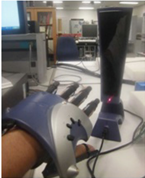
Fig. 7 P5 data glove for controlling the robotic hand
