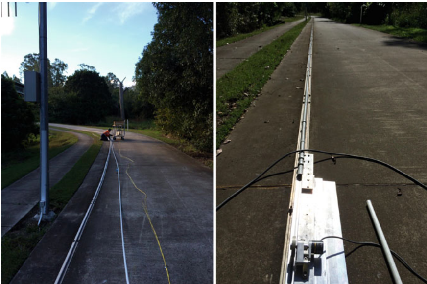
Fig. 5 Sensor wand testing on surveyed track
