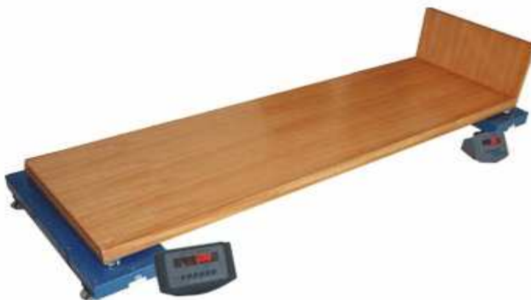
Fig.4 Traditional balance board measuring device
