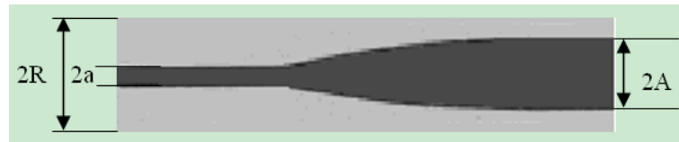
Fig.5 Schematic of the TEC fiber
