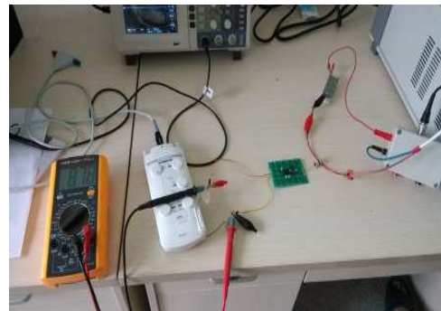
Fig.8 The WPT experiment system of a pacemaker
