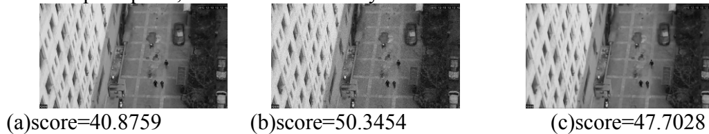
Fig.2 (a) a pristine image (b) an image with noises (c) a blurred image
