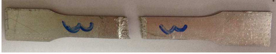
Fig5. The specimen and tensile fracture location
