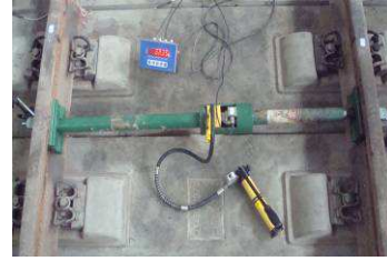
Fig.2 The photo of fastener's lateral stiffness test
