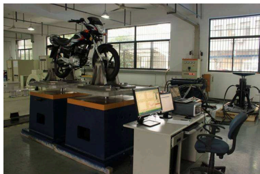
Figure 5. 2-axis random test system
