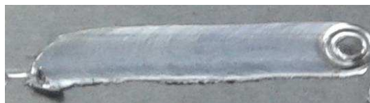
Fig.4 Surface appearance of Aluminum joint prepared by FSW
