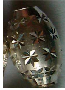
Fig. 10. The machined “米” pattern
