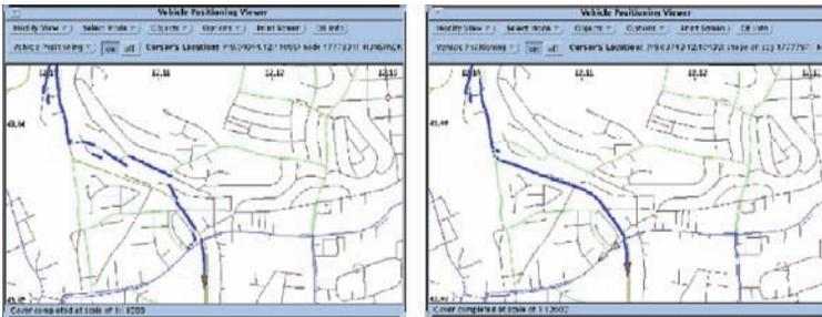
Fig. 8.8. Test drive B without (*left*) and with (*right*) pattern recognition
