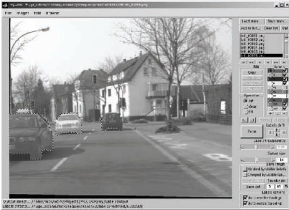
**Fig. 9.4.** myLabel – a tool for labeling video sequences. The labeling is similar to what is done in graphical editors like Photoshop or Gimp. Each label mask is represented by a separate layer with its own color (on the figure instead of colors we have used contours). The user can easily edit label masks in a pixel-wise manner as well as change their colors, transparencies and visibilities. myLabel allows semi-automatic labeling by interpolating the labels between two labeled frames
