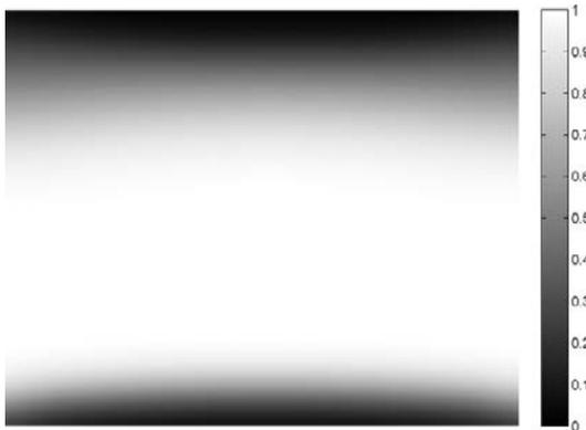
**Fig. 9.9.** Matrix  $M$ , masking regions of possible IMO appearance in a frame. This matrix has been chosen heuristically based on the logical assumptions that in normal circumstances IMOs are not supposed to appear “in the sky” or beneath the ego-vehicle
