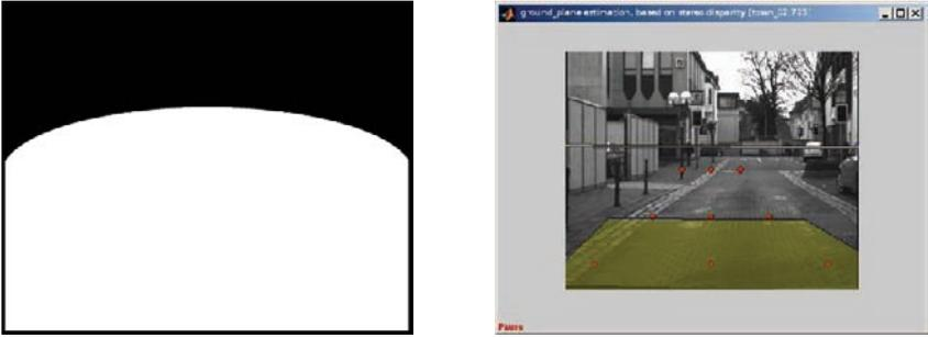
**Fig. 9.11.** (Left) Predefined road mask. (Right) Example of the ground plane estimation. Red points represent points used for ground plane estimation (see text)
