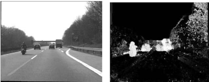
**Fig. 9.5.** (Left) Frame number 342 of motorway3 sequence. (Right) Matrix  $I$ , output of the motion stream for the same frame. Value  $I(x, y)$  is defined as probability of pixel  $(x, y)$  being part of an IMO
