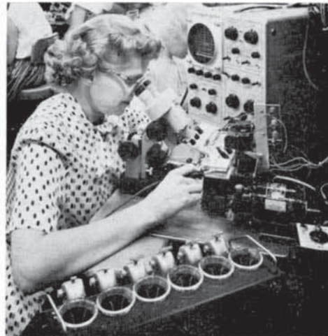
Testing of electrical characteristics of individual transistor dice (each smaller than a pinhead) must be done under a microscope. This is one of many testing procedures along the transistor production line.
