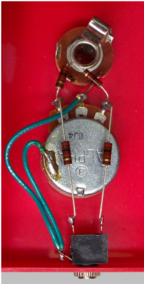
Figure 7-4. Sound card audio interface wiring (II)
