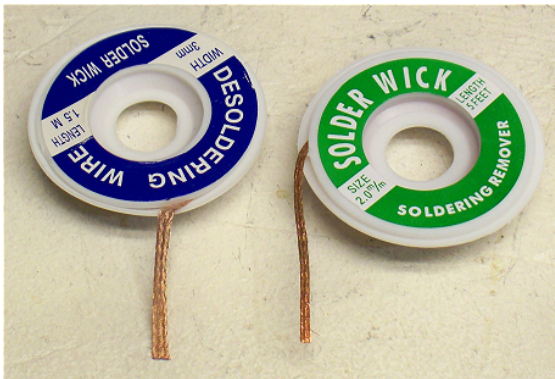
Figure 2-16. Two widths of desoldering wick
