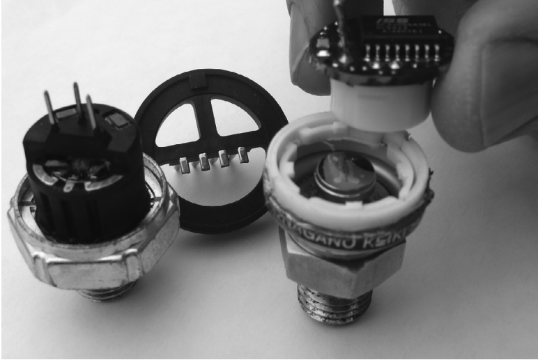
4.15 The interior construction of stainless steel diaphragm pressure sensors.
