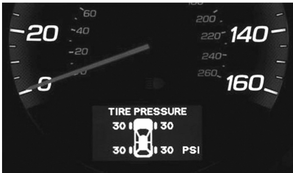
3.5 Typical display of TPMS systems with localization.
