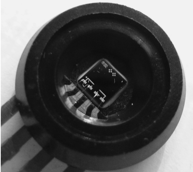
4.14 A plastic packaged silicon pressure sensor.
