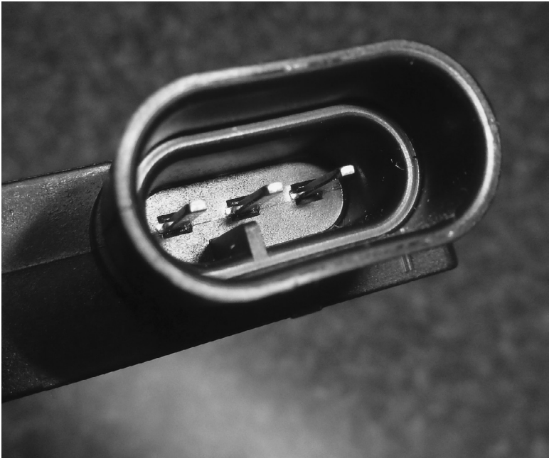
4.16 Three pin connector on an automotive MAP sensor.
