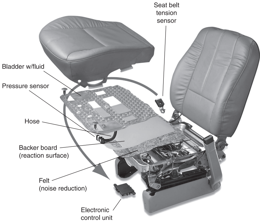
1.12 Delphi's 'Passive Occupant Detection System - B' (Figure is property of Delphi and used with permission).
