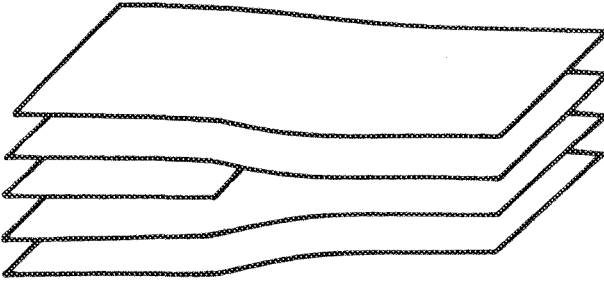
Fig. 11.2. Structure about an edge dislocation.
