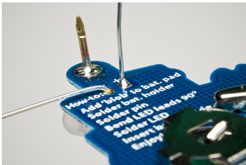
Figure 2-20. A good solder joint
