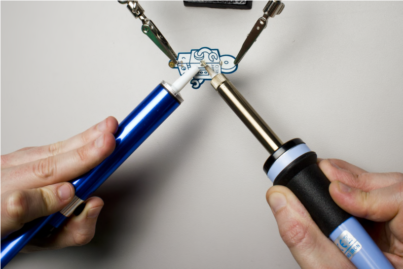
Figure 3-4. Using the solder sucker
