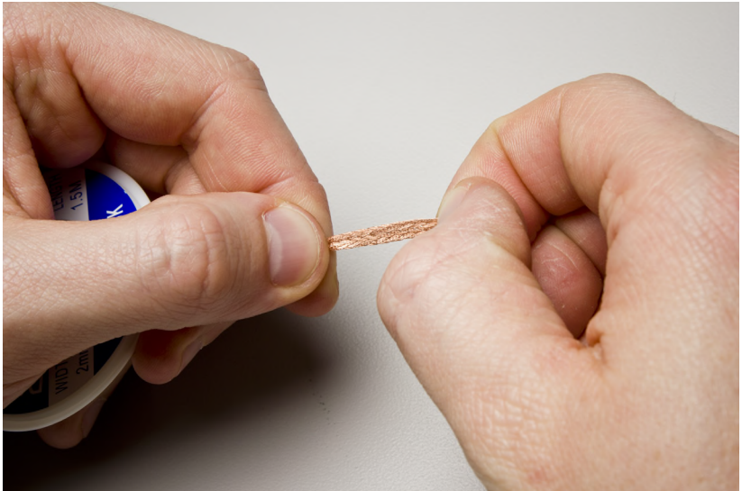
Figure 3-1. Pulling out some wick
