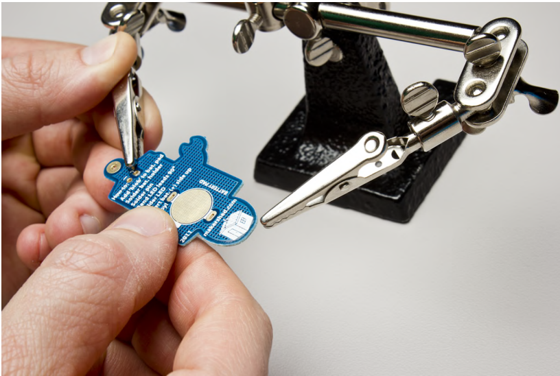
Figure 2-2. Holding a PCB in the helping hands
