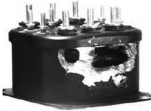
Figure 12.3 A hermetic relay whose failure is suspected to be caused by Sn whisker-induced metal vapor arc. (Reprinted with permission from the NASA Electronic Parts and Packaging (NEPP) Program [5]).
