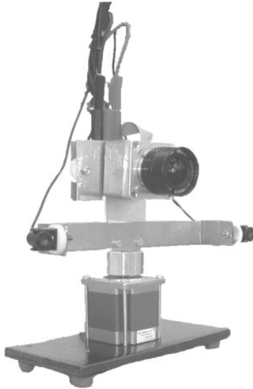
Figure 5.11 Transducer fixture. Camera and two ultrasound transducers are attached to stepper motor shaft.
