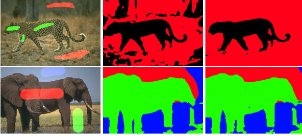
Fig. 2. Original image (first column). Segmentation using: just color distribution (second column) and with multiple clues (last column).
