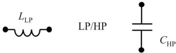
Fig. 14.10 Low-pass to high-pass transformation of a series inductor
