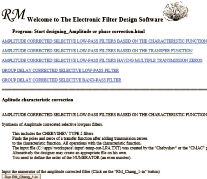
Fig. 5.2 Part of the screen seen by the designer in the amplitude or phase correction part of the design process
