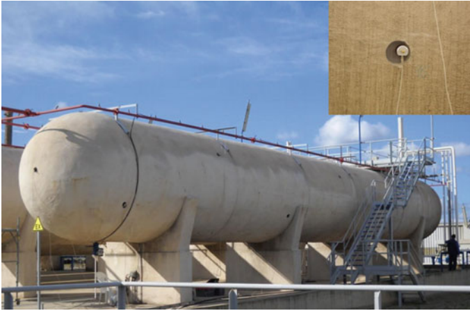
Fig. 3 AE method on a tank
