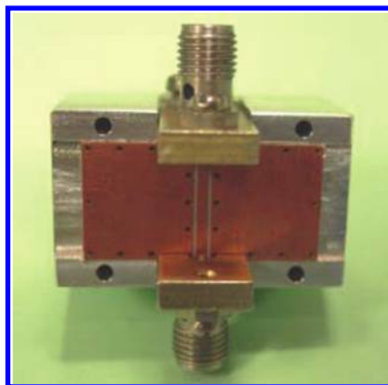
FIGURE 3.34 “Thru” calibration test fixture—top view.
