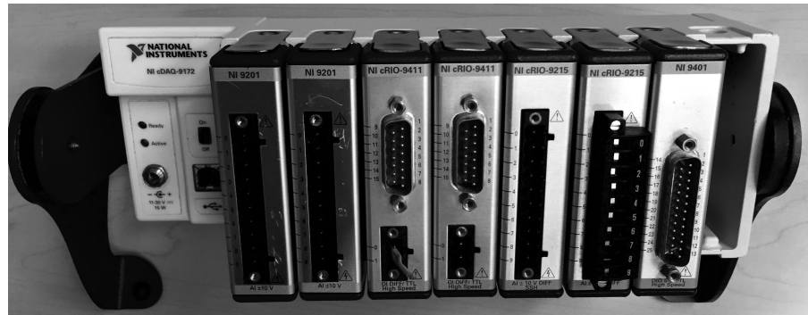
Figure 8.9 Typical data acquisition hardware (NI cDAQ-9172)
