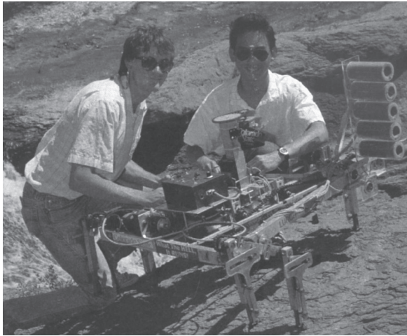
(a) "Lurch"—Scotch yoke mechanism leg design (1989)
