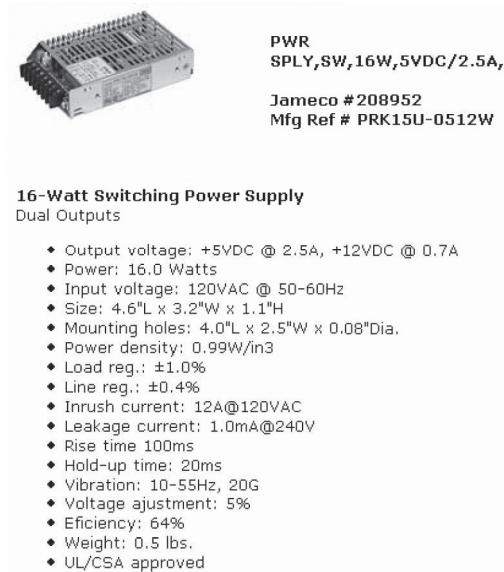
Figure 7.25 Specifications for an example closed-frame power supply.
