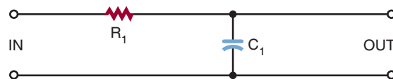
FIGURE 15-9 Lagging output phase-shift network. The voltage across the capacitor lags the applied voltage.
