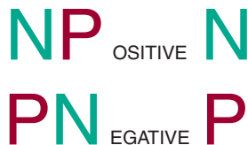
FIGURE 22–9 How to remember the polarity of the collector voltage.
