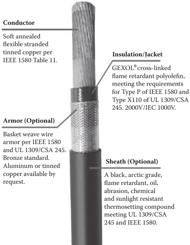
FIGURE 6.1 Single-conductor, 2-kV class power cable showing strands, insulation jacket, and outer sheath/shield. (From Gexol-insulated cable, a product of AmerCable, Inc. With permission.)
