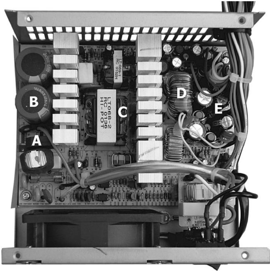
FIGURE 13.13 Switchmode power supply interior packaging (ATX Inc.).
