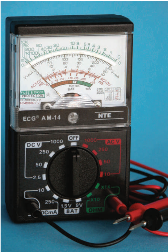
FIGURE 22-1 Analog meter used for AC measurements.
