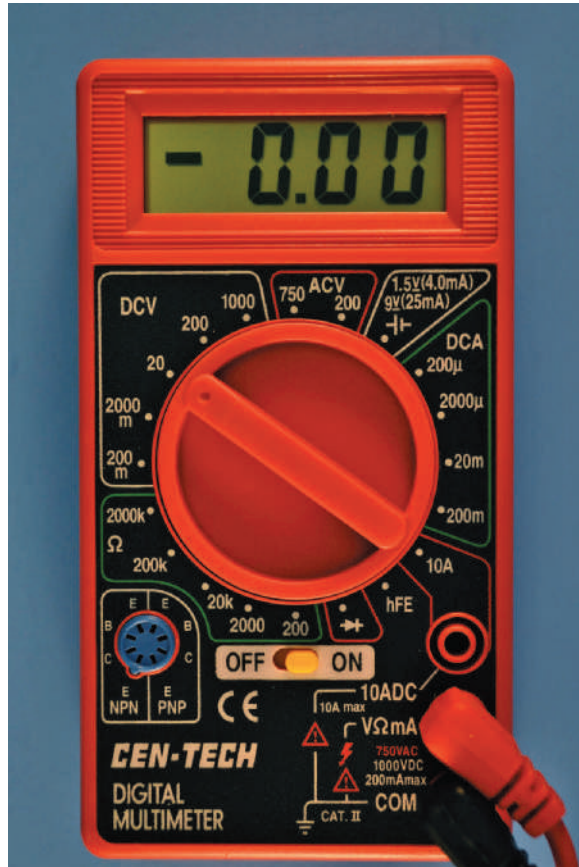
FIGURE 22-2 Digital meter used for AC measurements.
