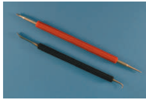
A. Spudgers for lifting wires and aligning leads.
