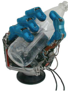
Fig. 9. The DLR hand with four dexterous fingers and a self-contained structure
