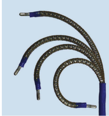
Fig. 4. A continuum manipulator with tendon actuation
