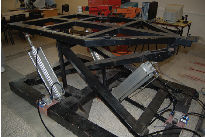
Fig. 1. SIMPRO 3DOF pneumatic driver simulator parallel platform
