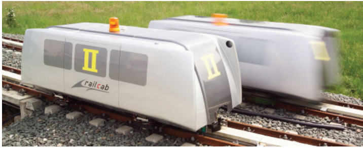
Fig. 1. Autonomous shuttles traveling on the NBP test track at the University of Paderborn
