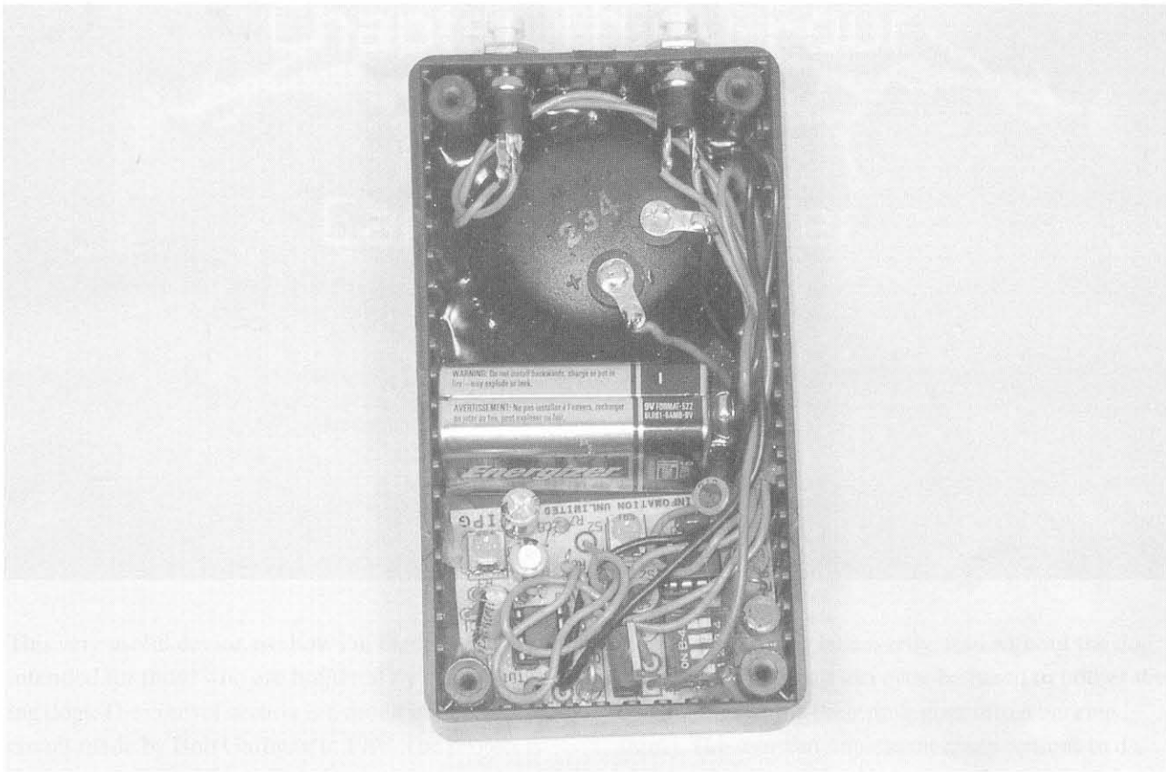
Figure 33-6 Final assembly into EN1 enclosure
