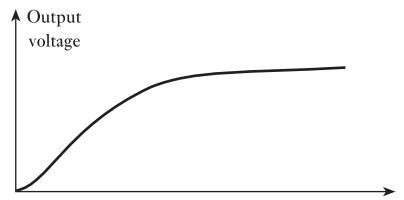
Fig. 28.9 Response with critical damping
