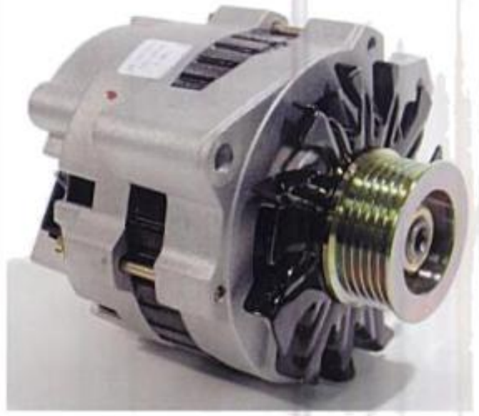
This Delco Remy alternator features a test hole at the back of the alternator. Just stick a pocket screwdriver or Allen wrench into this hole and the alternator will full field. Courtesy of CARQUEST Auto Parts
