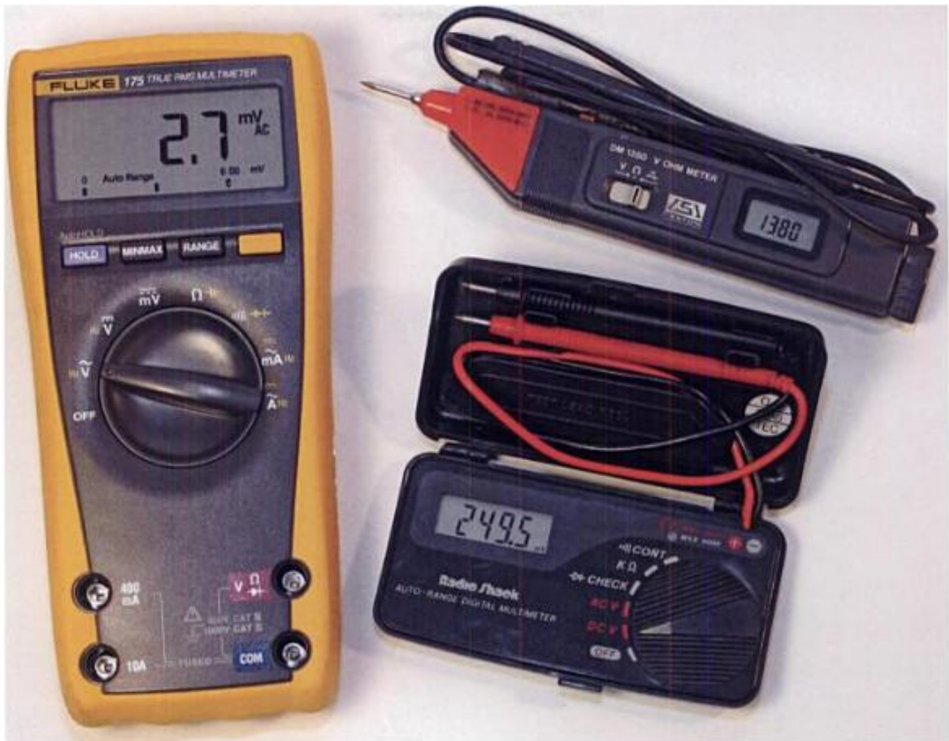
The Fluke 175 digital multimeter (left) has a bar graph feature not found on less expensive digital meters. Radio Shack's pocket digital multimeter (lower right) has more functions and gives more bang for your buck than other meters costing several hundred dollars a few years ago. Courtesy of Fluke Corporation
