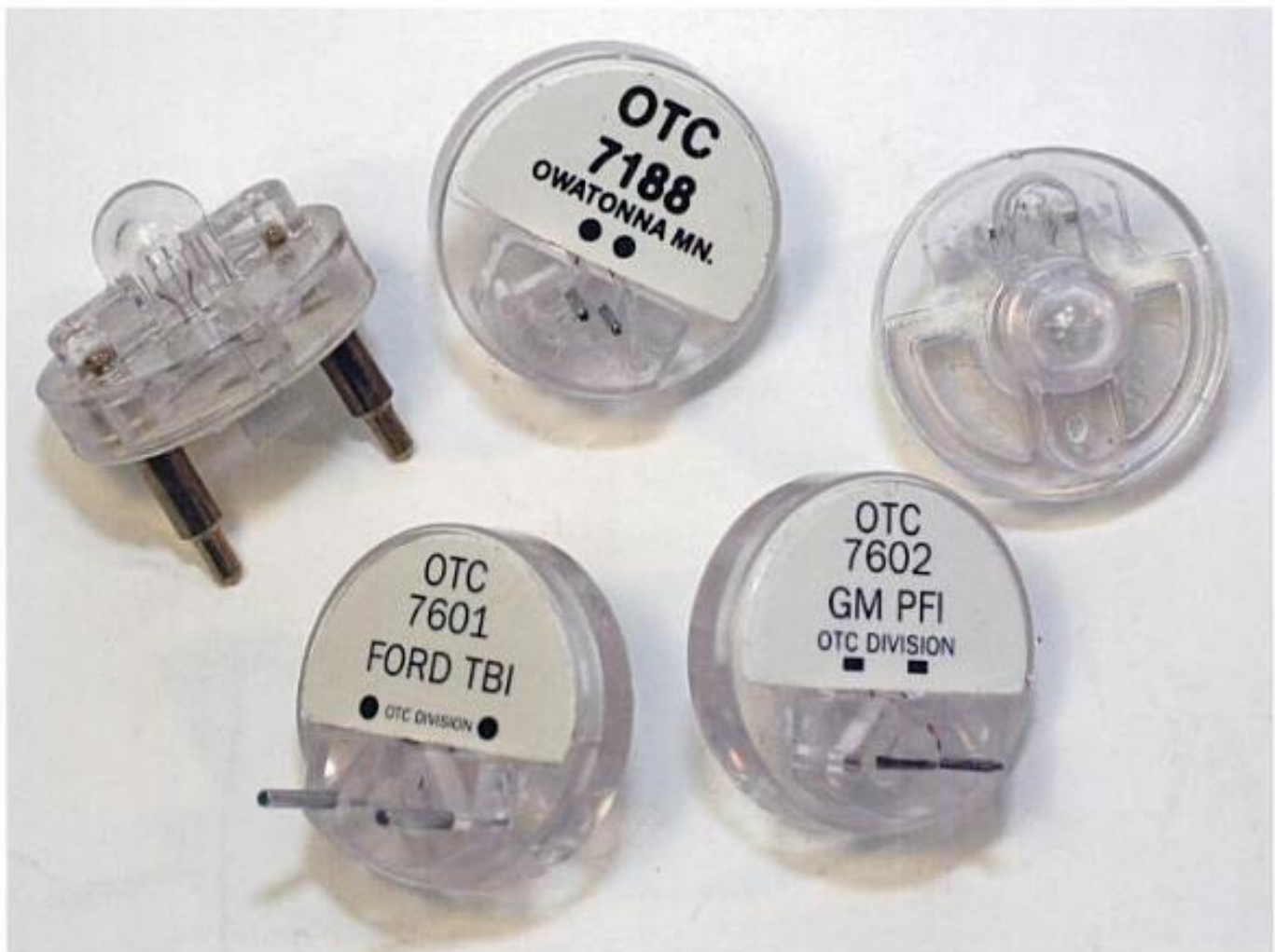
Each of these Noid lights fit different fuel-injection wiring harnesses. When connected, they flash whenever an injector pulse from the ECM is present. Courtesy of SPX/OTC
