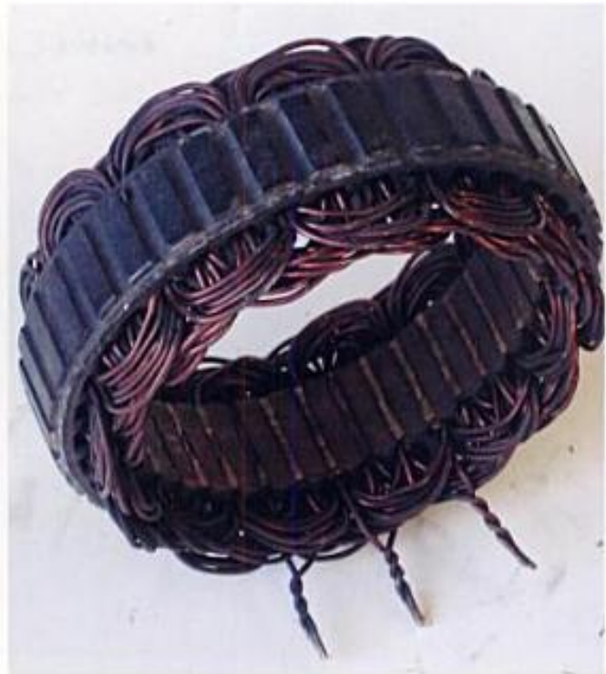
The alternator's stator is made up of three separate coils. The rotor spins inside the stator, inducing voltage and current into the stator windings (or coils).
