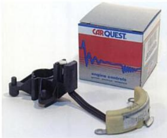
This hall-effect switch (left) is for a Ford vehicle. The white plastic connector (right) connects the switch to the ignition module. Courtesy of CARQUEST Auto Parts
