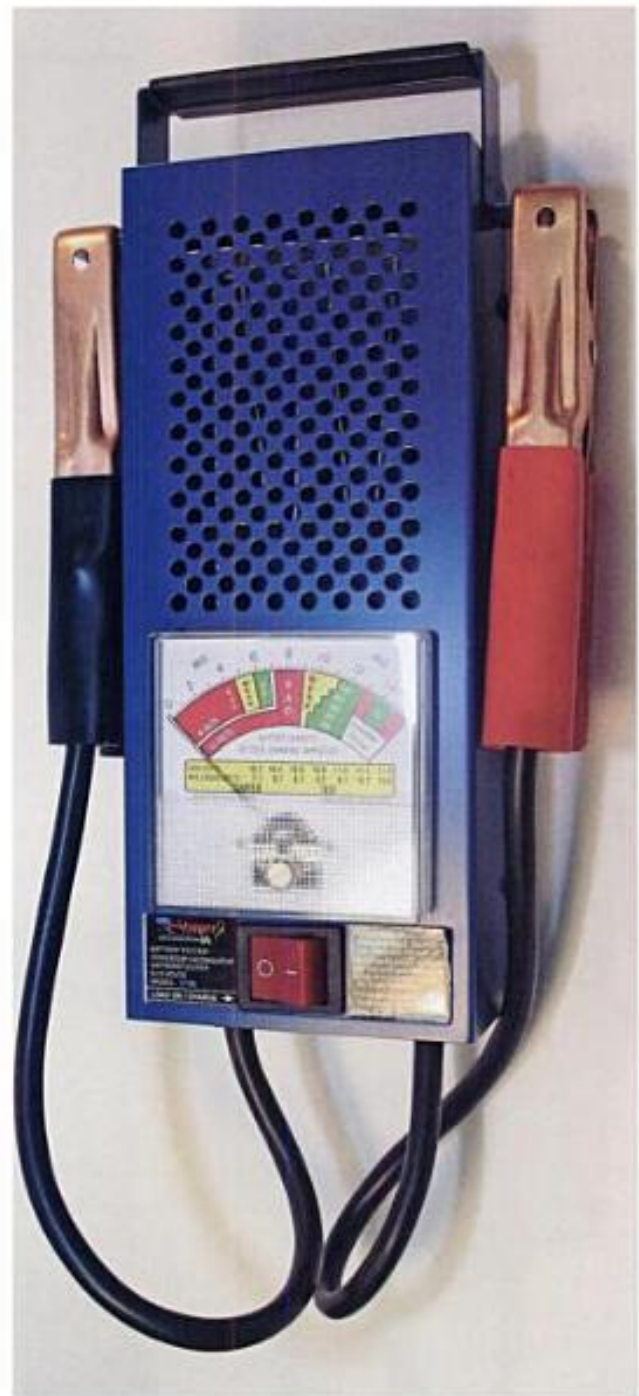
An OTC 3180 Stinger battery tester pulls a 100-amp load during battery testing. Hand-held battery testers are more convenient than using the engine's starter motor. Either a 6-volt or 12-volt battery can be tested. Courtesy of SPX/OTC
