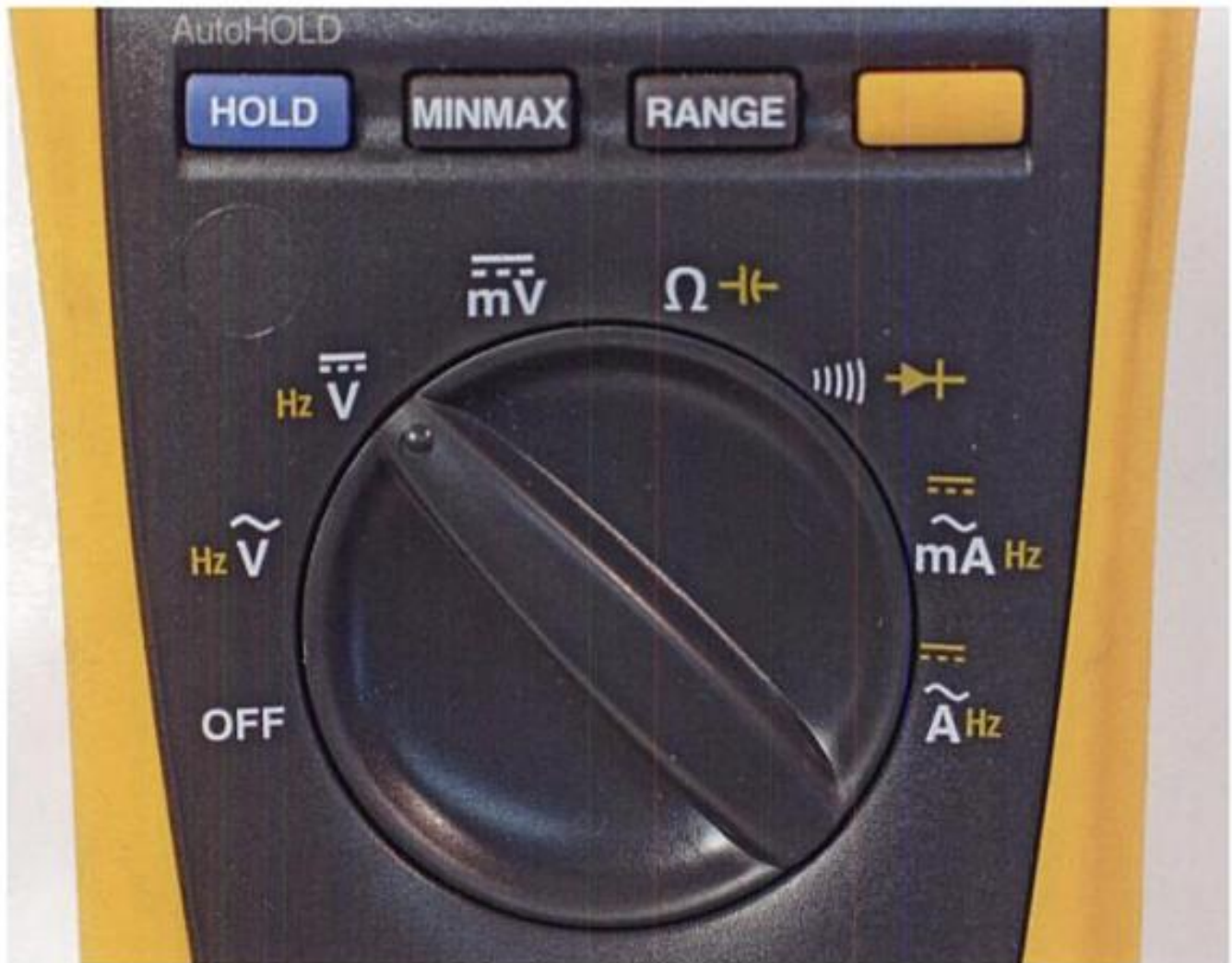
In addition to reading volts, amps, ohms, and frequency, this Fluke Series 170 multimeter has "Hold" and "MinMax" features. The yellow button switches the meter's reading modes between white and yellow lettered dial functions. Courtesy of Fluke Corporation
