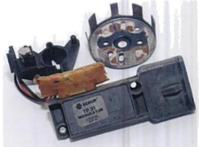
Shutter blades (top right) inside the distributor pass between the hall-effect switch (on the left) and a magnet. The hall-effect switch is connected (with a brown connector) to the Thick Film Ignition (TFI) module that is mounted on the side of the distributor.
