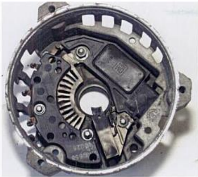
An internal voltage regulator (upper right) is on this GM alternator. Diodes are located on the left; slip ring brushes are at the bottom.
