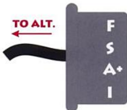
Fig 5-13. Full fielding is accomplished in the same manner for both types of Ford's charging systems. To full field, jump terminals F through A+. The alternator should produce amperage within 10 percent of its rated output capacity.
