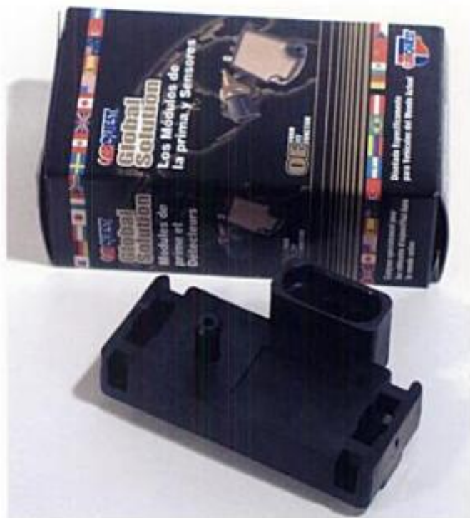
This GM MAP sensor has a nipple connecting the sensor (via a vacuum hose) to the engine intake manifold. These sensors produce a voltage signal to the ECM. Courtesy CARQUEST Auto Parts
