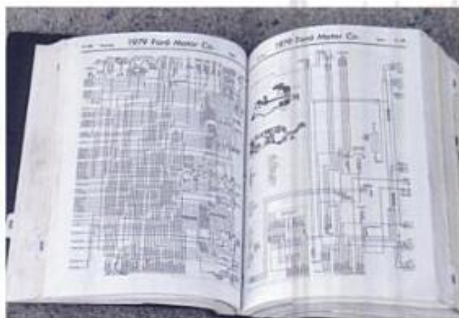
Many automotive technicians with years of experience prefer to use a book version of wiring diagrams. However, today, most wiring diagrams intended for professional use can be found on a CD or DVD. A technician can read them on a computer monitor and print out, one page at a time, as needed. Courtesy Scott's Speed Shop and Mitchell 1.
