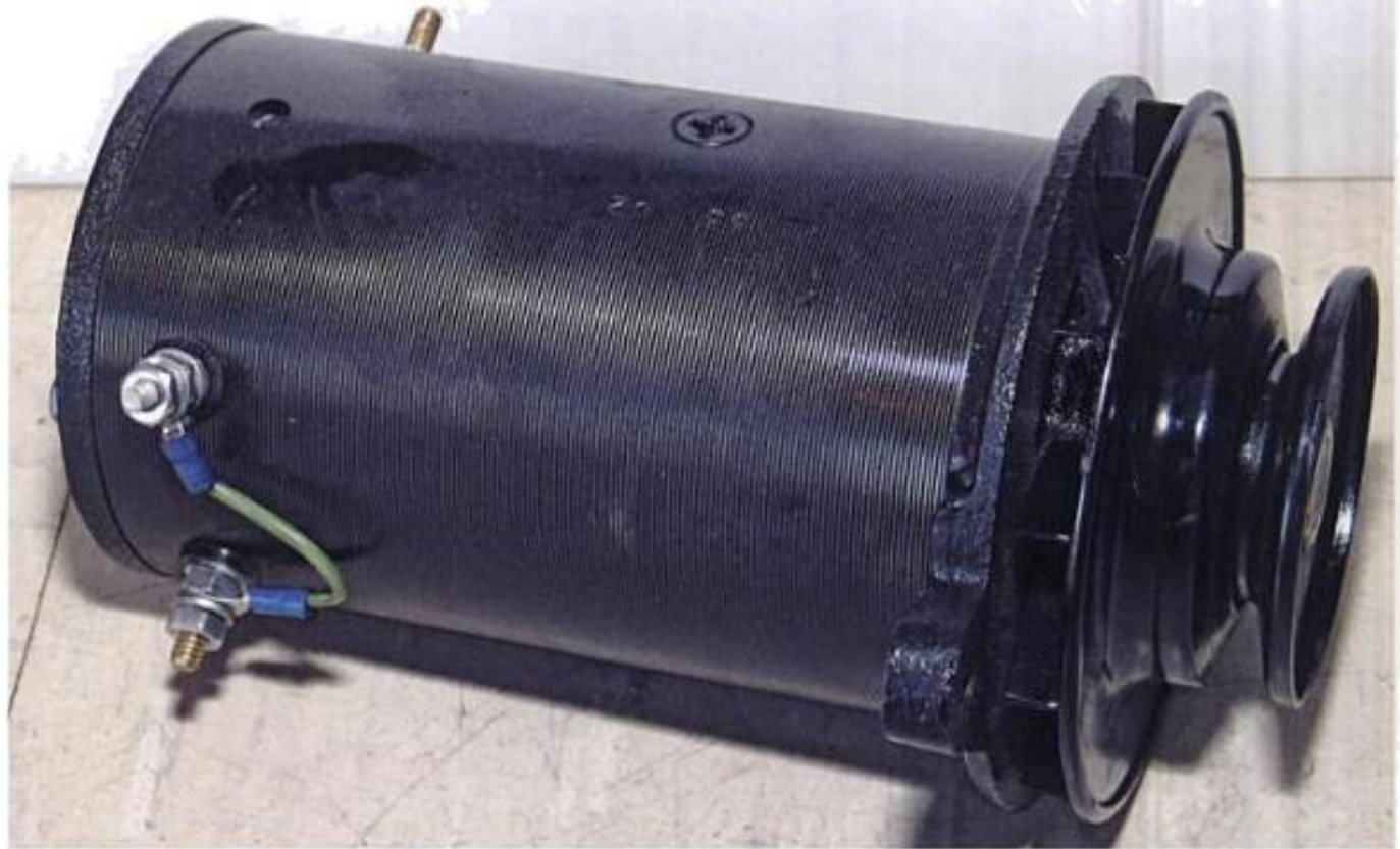
DC generators are limited in current-producing capacity because all amperage must pass through the generator brushes. Most generators are only capable of producing about 25 to 40 amps—not enough for modern vehicles. Courtesy of Auto Electric, Inc.
