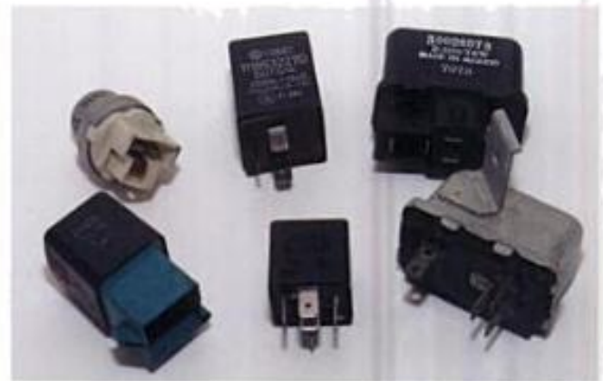
Automotive relays come in all shapes and sizes, but they all basically operate the same. Some late model vehicles use as many as 30 relays or more.
