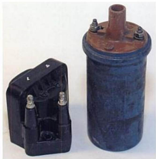
The difference between the DIS coil (left) and a conventional coil is that the DIS coil's secondary windings are not connected to the primary circuit. This design causes the spark produced by a DIS coil to go to the other side of the secondary windings and not the battery ground.
