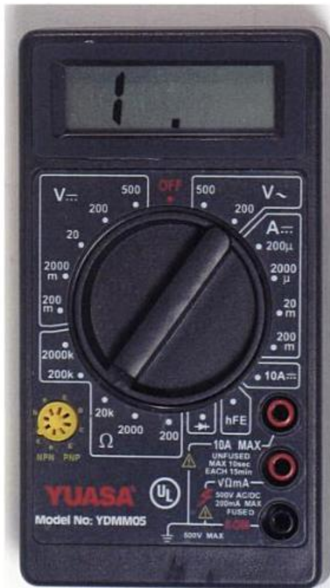
Before reading voltage or resistance, this Yuasa digital meter without an auto-ranging feature must be set to the correct scale. Courtesy Yuasa Battery
