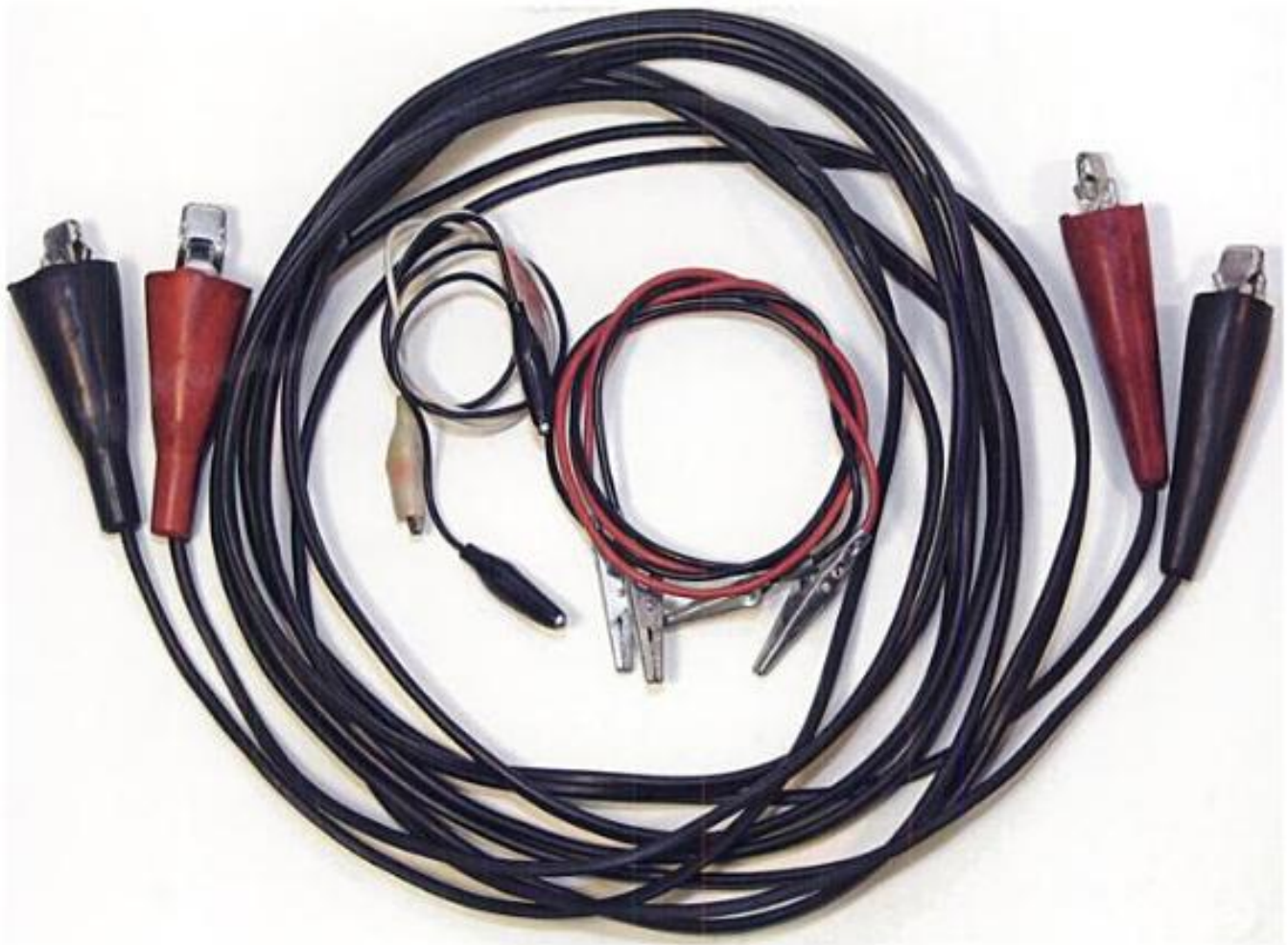
A person can never have too many jumper wires. They come in all different sizes, as shown here. The large set of jumpers was homemade using 14-gauge lamp cord; it comes in mighty handy for getting power from the front to the back of a vehicle or trailer.
