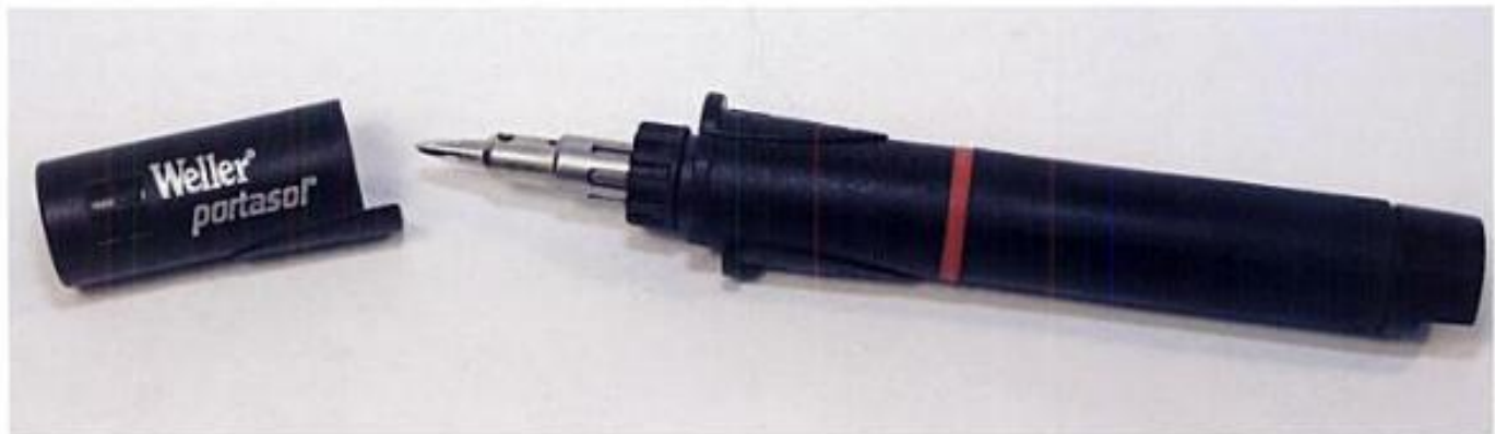
Weller's Portasol—a completely portable, butane-powered soldering iron. This tool is convenient and invaluable when working on trailer wiring, under the dash, at the racetrack, or on those dreaded roadside repairs. Heat is adjustable and ignition is via a piezoelectric system—just flick the ON switch. The tool can be charged with butane using the same canisters that fill cigarette lighters. One fill-up lasts several hours—more than enough time to solder entire wiring harnesses. Courtesy of Weller
