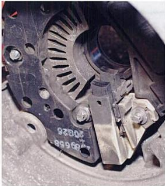
With the rotor removed, the alternator brushes can be seen. They are made from carbon and are spring-loaded so they will make contact with the rotating slip rings when the alternator operates.
