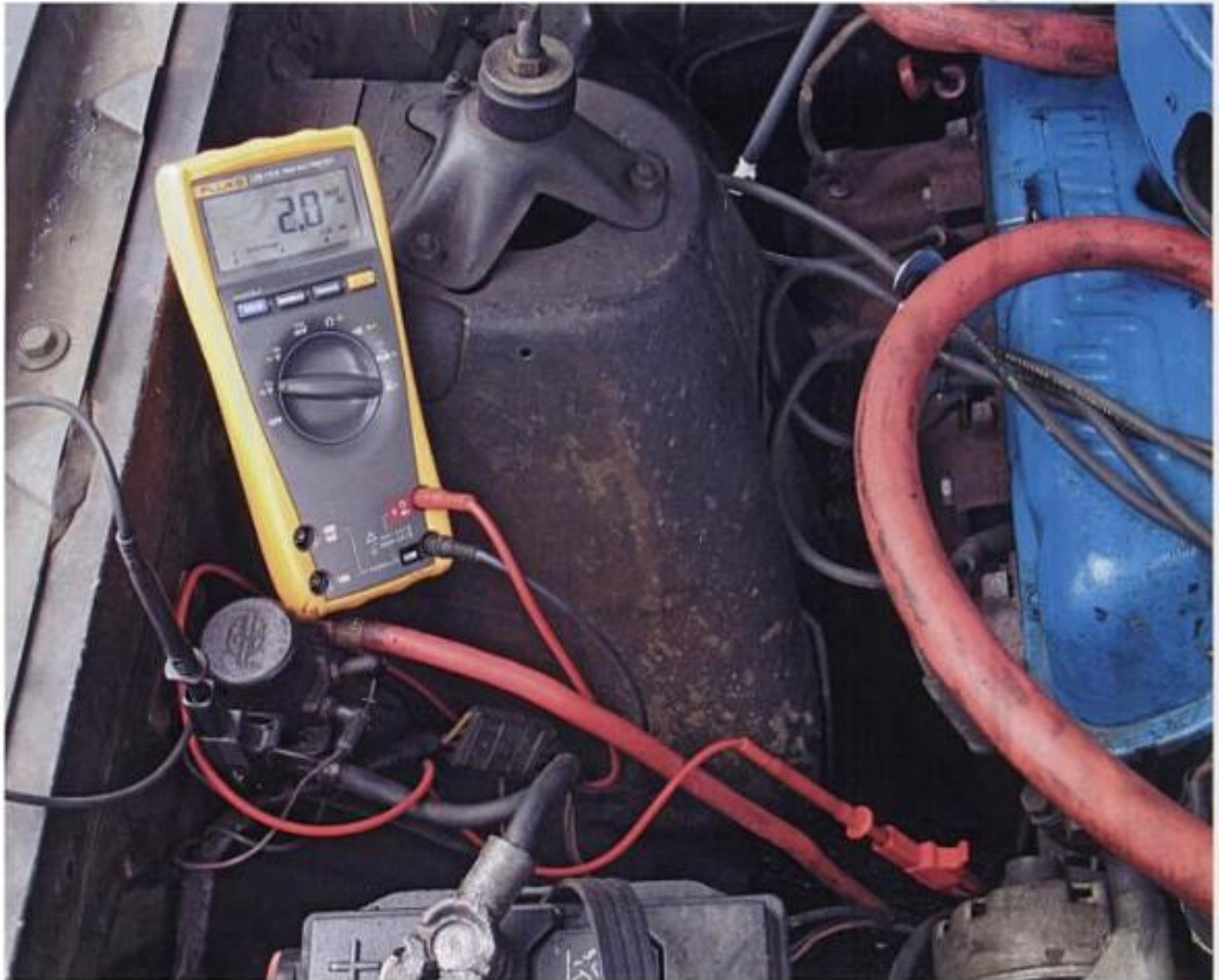
The red lead is connected to the big wire on the back of the alternator. The black lead is connected to the positive battery post. With all electrical accessories on and the engine holding at 2,000 rpm, the voltage drop on the positive power side of the alternator circuit will be displayed.
