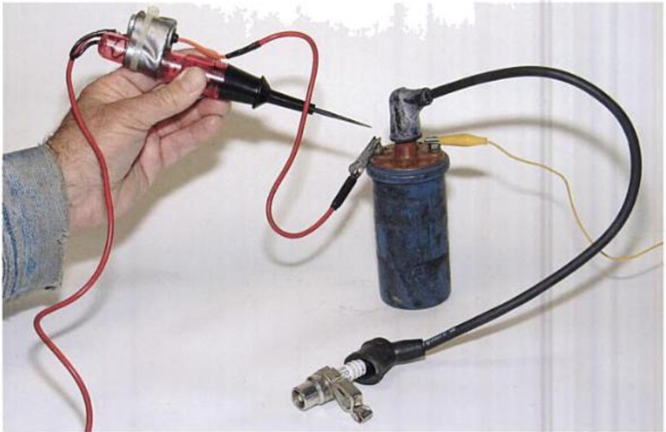
This ignition coil is being bench-tested. The yellow wire is 12 volts and the wire coming out of the coil tester goes to ground. When the pointy end of the coil tester is tapped on the negative coil terminal, a spark is produced.
