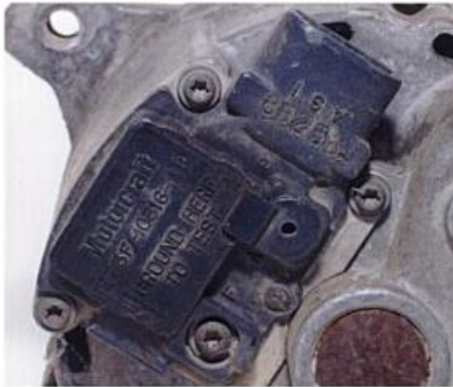
This Ford IAR alternator uses an internal voltage regulator. "Ground here to test" is marked on the regulator. To full field the alternator the F terminal on the regulator is grounded.
