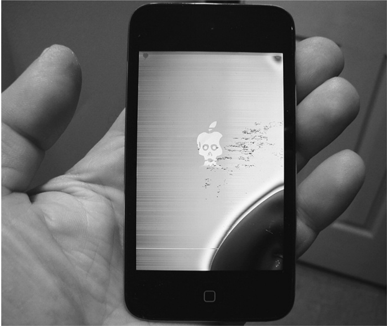
FIGURE 15-14 Ruined LCD on an iPod with the same construction as a phone.
