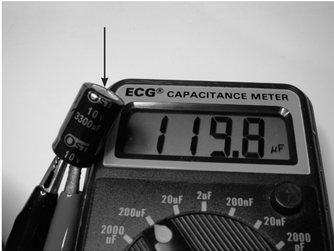
FIGURE 7-2 Bulging 3,300 \mu\text{F} electrolytic capacitor with greatly reduced capacitance.
