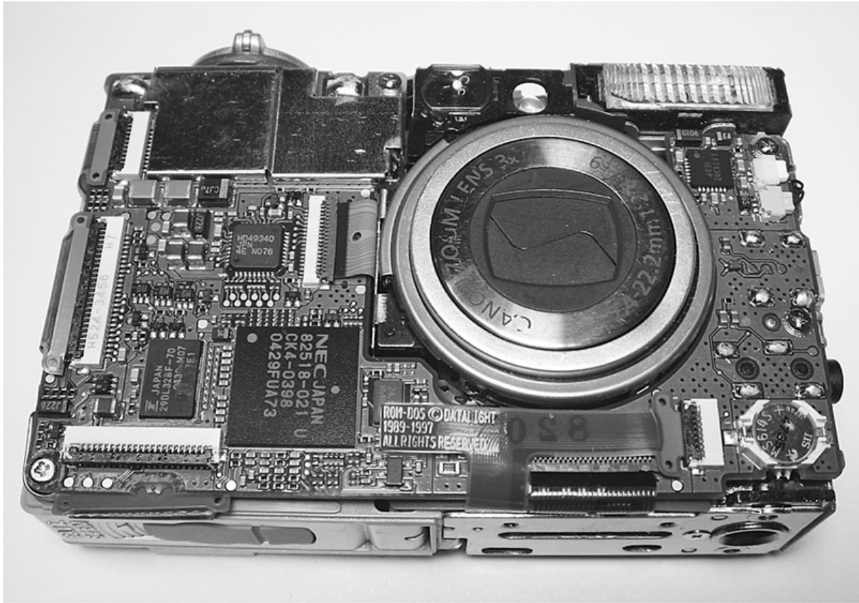
FIGURE 9-6 Inside a digital camera.
