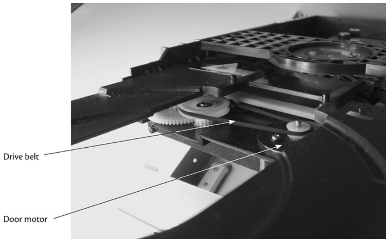
FIGURE 15-4 Door mechanism with belt on underside of platform. The leaf switch is not visible.
