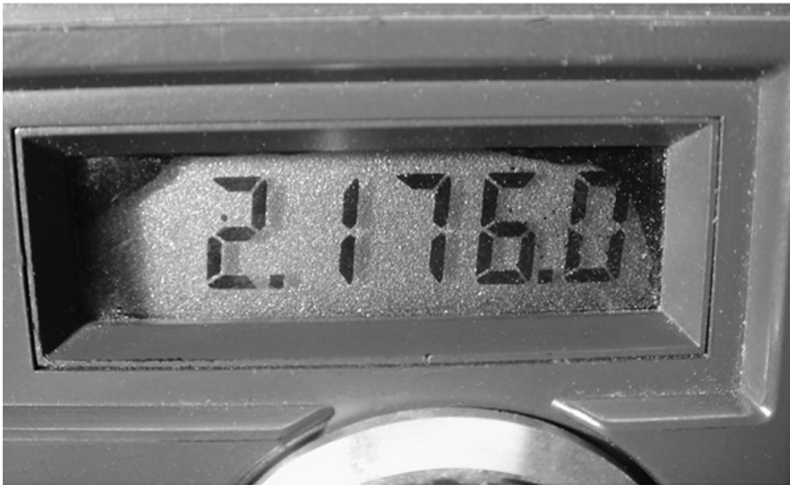
FIGURE 14-7 After a nice massage, this LCD isn't perfect, but it sure is more readable!
