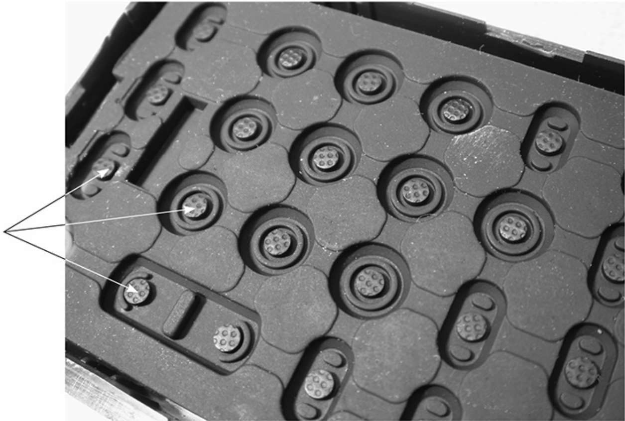
FIGURE 15-10 Conductive end of rubber buttons.
