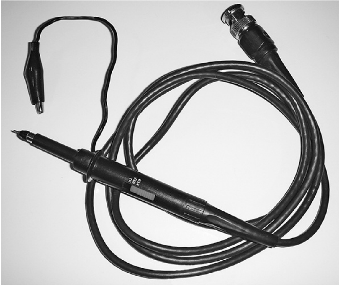
FIGURE 2-4 Oscilloscope probe, 10X/1X switchable.
