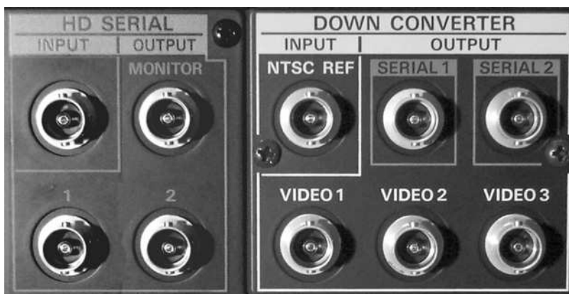
Figure 13.6 Down Converter on HD VCR
