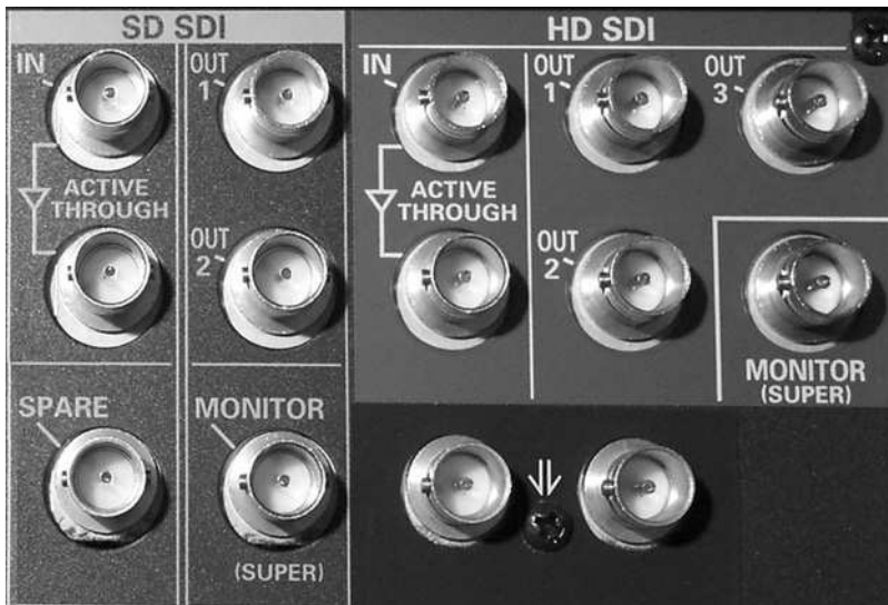
Figure 11.5 Serial Digital Interface (SDI)
