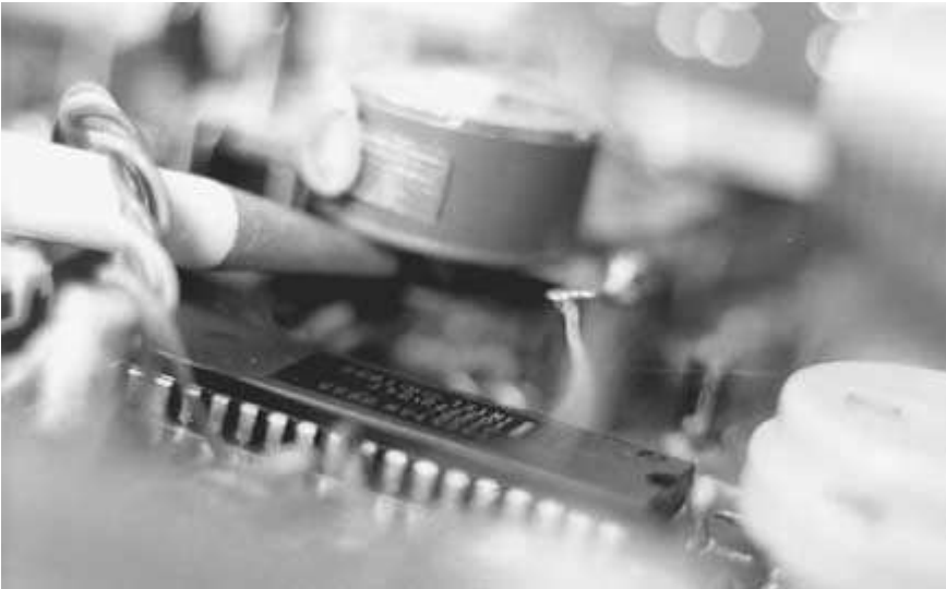
FIGURE 8-21 The LSI CPU or microprocessor found in an answering machine usually has 36 or 42 pins.
