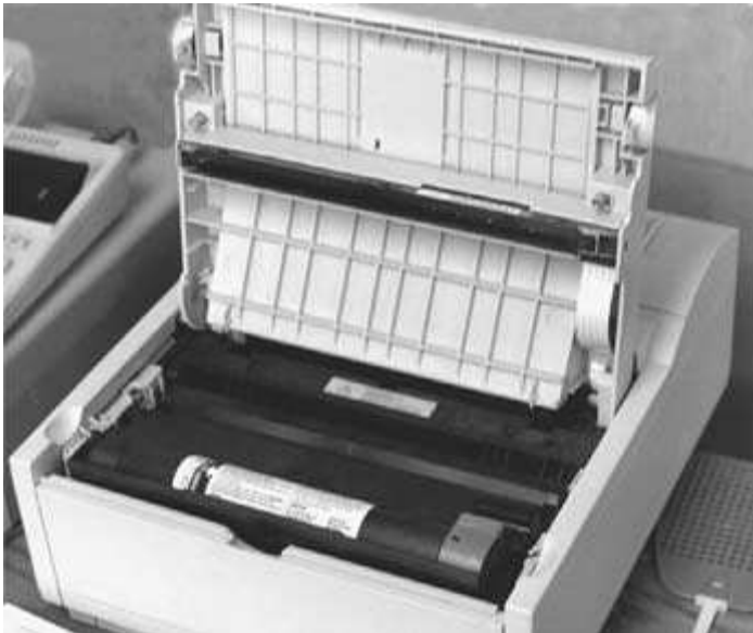
FIGURE 10-29 A laser copier with the cover tilted up so as to be cleaned or serviced.
