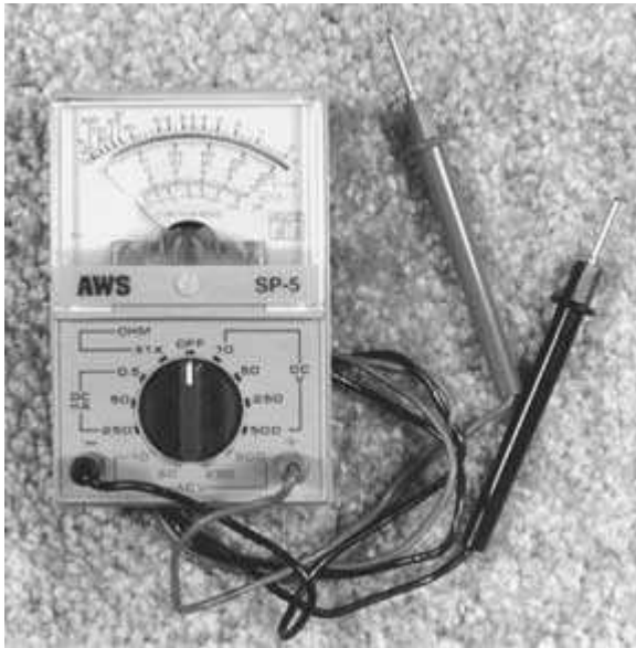
FIGURE 1-7 A small volt-ohm multimeter that is used to check resistance values in electronic equipment.
