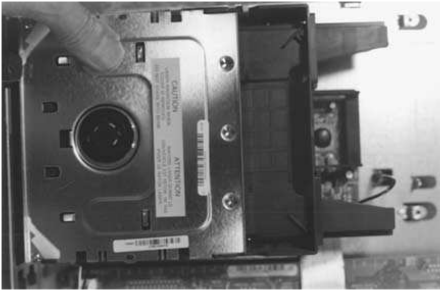
FIGURE 11-9 The tray has been removed from the DVD player to repair a problem with the tray slide not operating properly.
