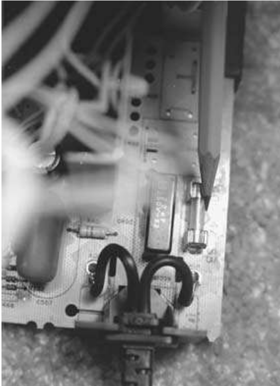
FIGURE 4-6 The main power clip-in fuse used in some TV sets.
