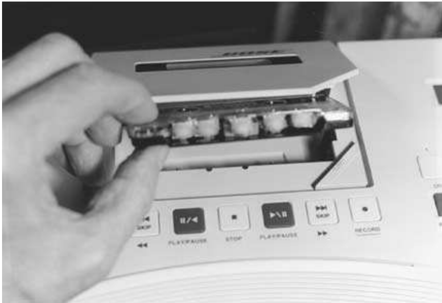
FIGURE 2-35 The Trackmate cleaning cassette has 32,000 absorbent, flexible cleaning fibers.
