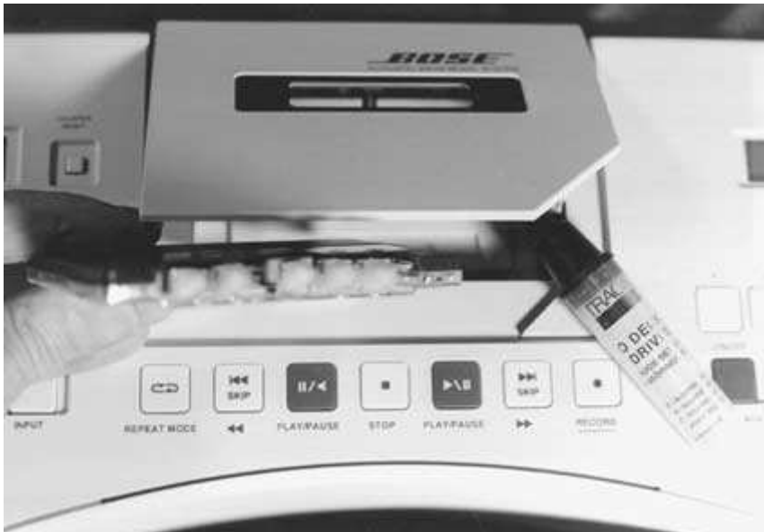
FIGURE 2-36 Cleaning fluid is being applied to the Trackmate fiber brushes.
