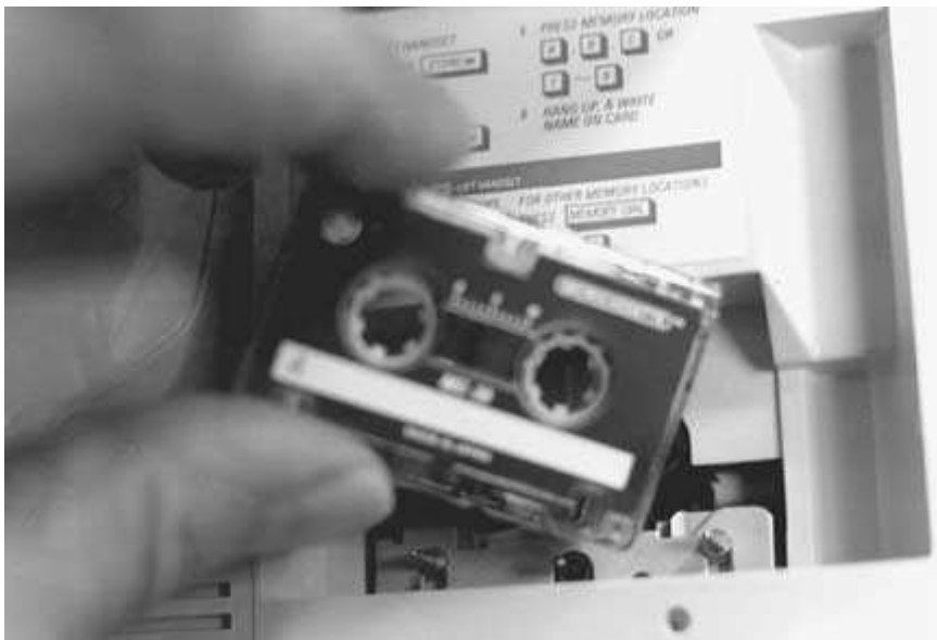
FIGURE 8-17 A cassette being inserted into the tape compartment of an older model answering machine.
