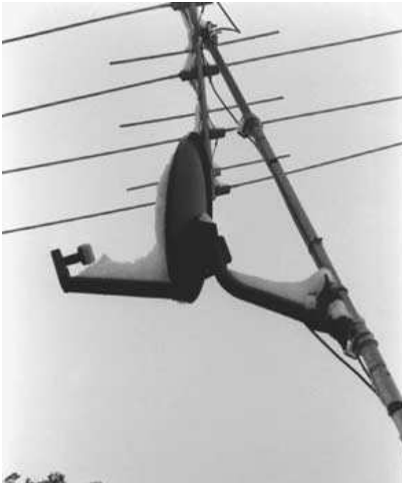
FIGURE 6-32 Snow or ice buildup on the dish can prevent DBS signal reception. A dish heater is available that will melt any ice or snow if you live in a northern climate.
