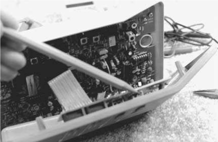
FIGURE 8-43 Clean dust and dirt from the switch contacts. Use a brush or a spray switch contact cleaner.
