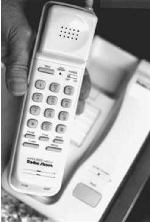
FIGURE 8-34 This cordless phone uses analog RF signals with frequency modulation on frequencies allotted from 46 MHz to 50 MHz.
