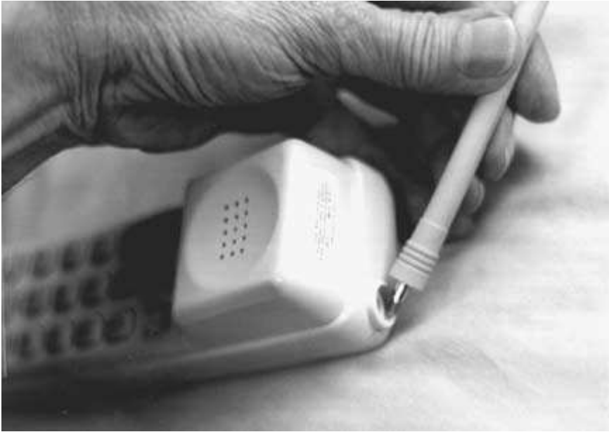
FIGURE 8-46 A new antenna is being replaced. Most older-model cordless phone antennas will screw in.
