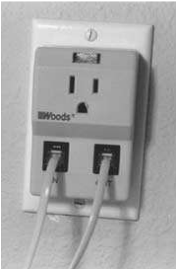
FIGURE 8-47 A telephone line-protection device can be easily plugged into an ac wall outlet. This provides good protection from spikes and lightning damage that can be coming into the phone line.
