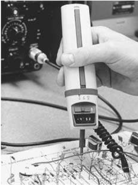
FIGURE 1-59 A small, easy-to-use, battery-operated, portable volt-ohm meter. Some cost $45 to $85.
