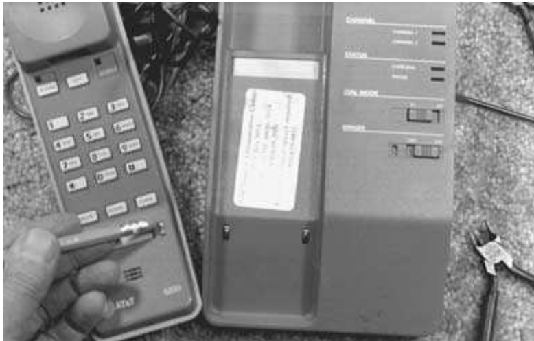
FIGURE 8-44 Clean these contacts if the battery will not charge or if the phone does not work, but gives you a beeping tone that indicates a low battery.
