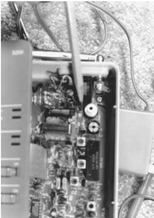
FIGURE 8-41 After the screws are removed, the covers will come apart.
