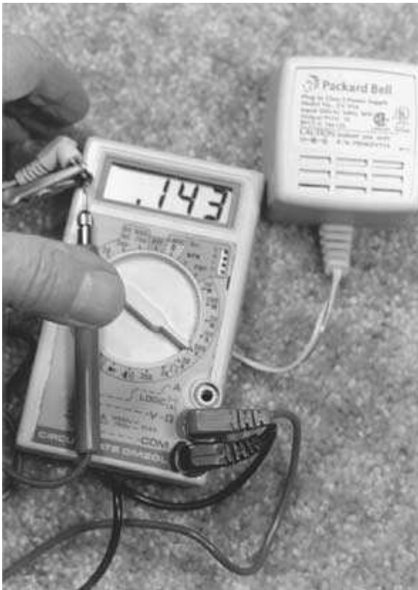
FIGURE 1-44 A digital multimeter is being used to check a “block-type” plug-in power supply.
