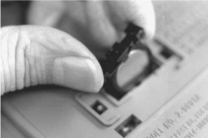
FIGURE 8-31 The small, thin battery used for chip memory is shown being replaced.
