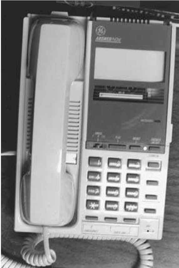
FIGURE 8-18 A typical stand-alone tape-type answering machine and telephone combination.
