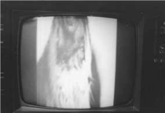
FIGURE 4-33 The picture (raster) is pulled in from both sides of the screen.
