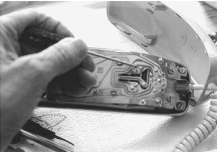
FIGURE 8-16 A PC board hairline crack is hard to locate, but can cause all sorts of phone problems.
