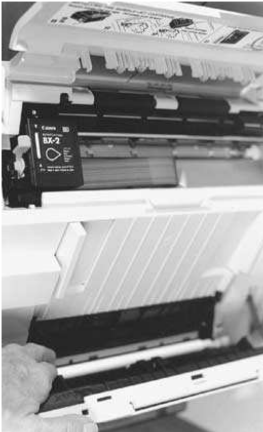
FIGURE 10-11 The BX-2 print head is shown on the left side. It moves to the right side on a carriage rod to print lines across the paper.
