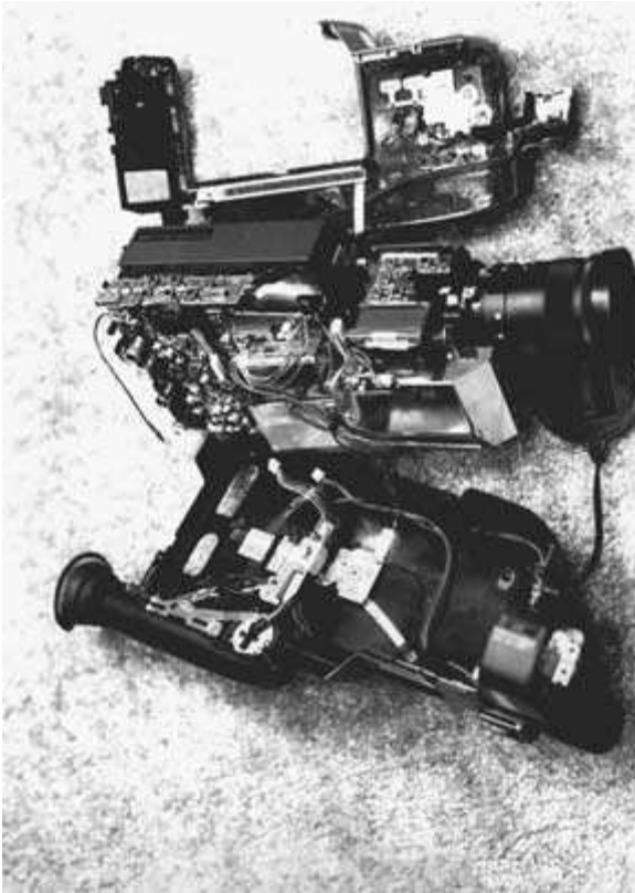
FIGURE 7-26 The Sony HandyCam camcorder split apart for cleaning, adjustment, or repairs.
