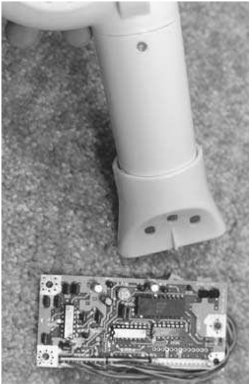
FIGURE 1-61 A hair dryer being used to heat one section of a PC board to locate an intermittent problem.
