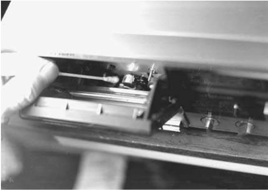
FIGURE 2-32 Use a cotton swab with alcohol to clean the tape record/play heads.
