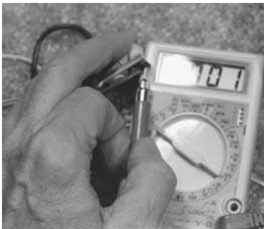
FIGURE 1-10 A digital ohmmeter being used to check a fuse.
