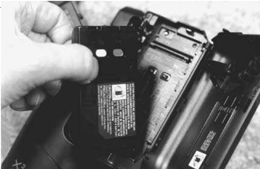
FIGURE 7-21 Be sure that the battery is installed properly and that the contacts are clean.
