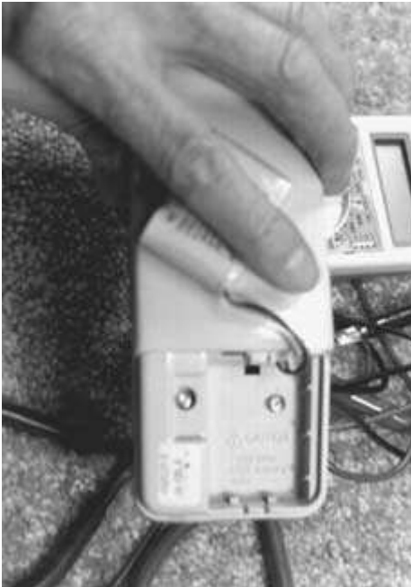
FIGURE 8-45 If the phone will not work, unplug the battery (small red and black wires). Wait 15 seconds and plug the battery back in. The phone should now be operational again.
