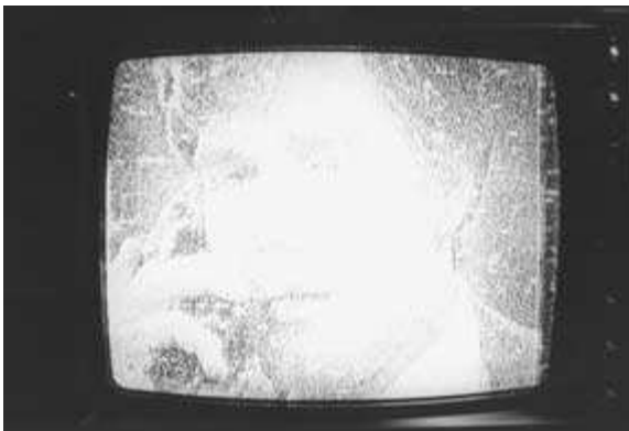
FIGURE 4-37 An out-of-focus or blurred picture symptom.
