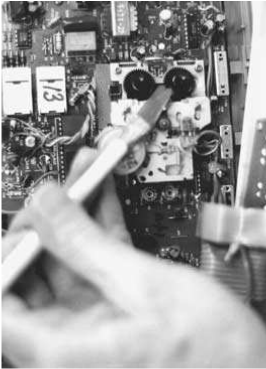
FIGURE 8-25 Use a small brush and alcohol to clean all tape recorder mechanical parts.
