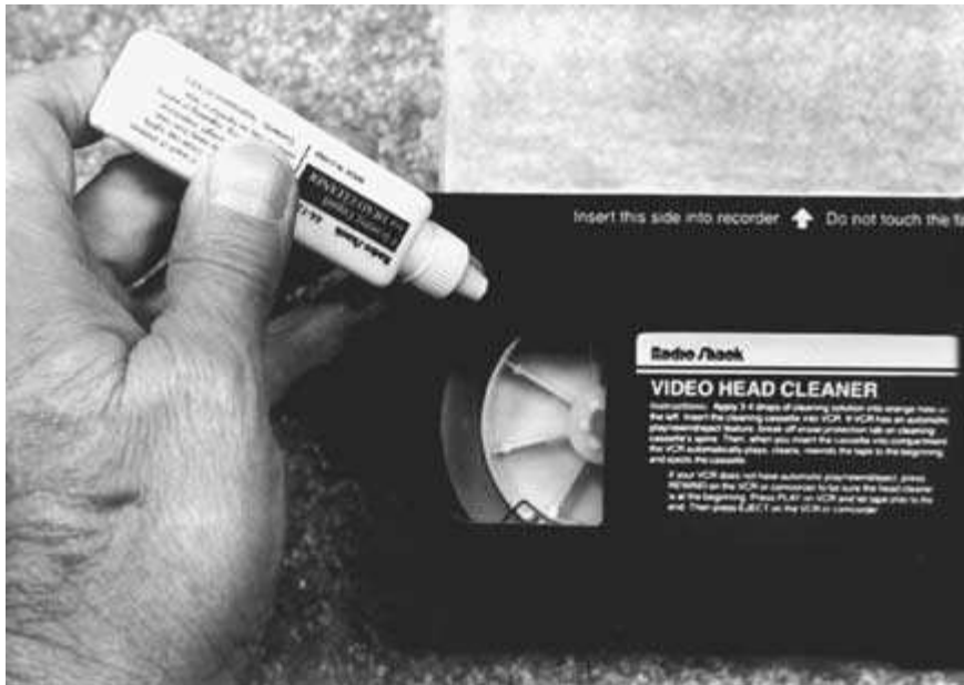
FIGURE 7-19 Cleaning fluid is being applied to a video head cleaner cassette.
