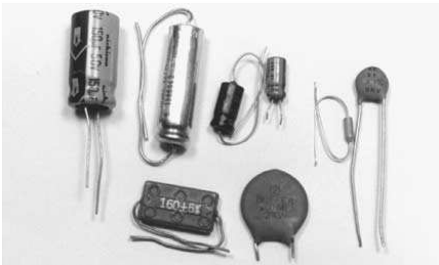
FIGURE 1-12 Disc ceramic capacitors are shown on the right side of the photo and tubular electrolytic capacitors are shown on the left side of photo.
