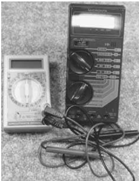
FIGURE 1-58 Some inexpensive digital volt-ohm meters that are very useful for electronic circuit repairs.
