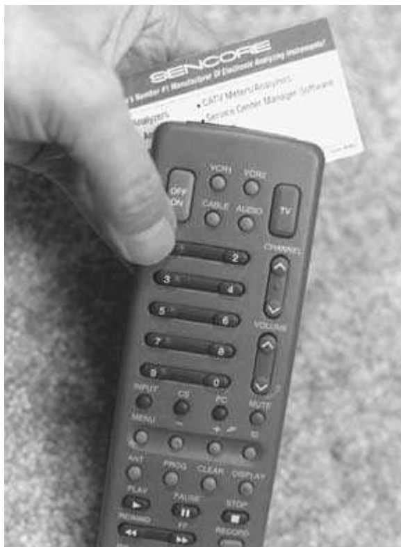
FIGURE 9-7 Testing a remote IR transmitter with an IR detection card.
