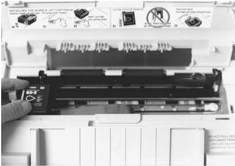
FIGURE 10-7 The print head and ink cartridge being replaced on the Canon model 1000 machine.
