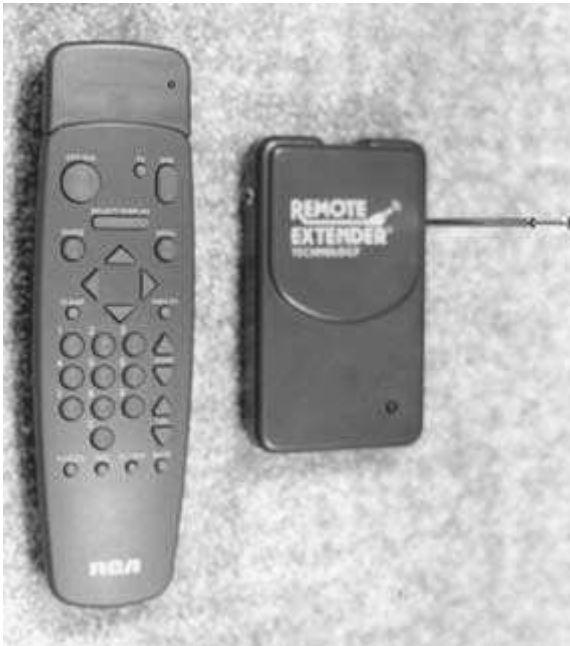
FIGURE 9-10 The Windmaster remote control DBS extender control unit on the front of the DBS control unit and the receiver unit.
