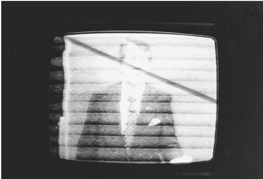
FIGURE 7-28 Nose bars (streaks that are caused by a very worn tape cylinder head drum) are shown going across the monitor screen.
