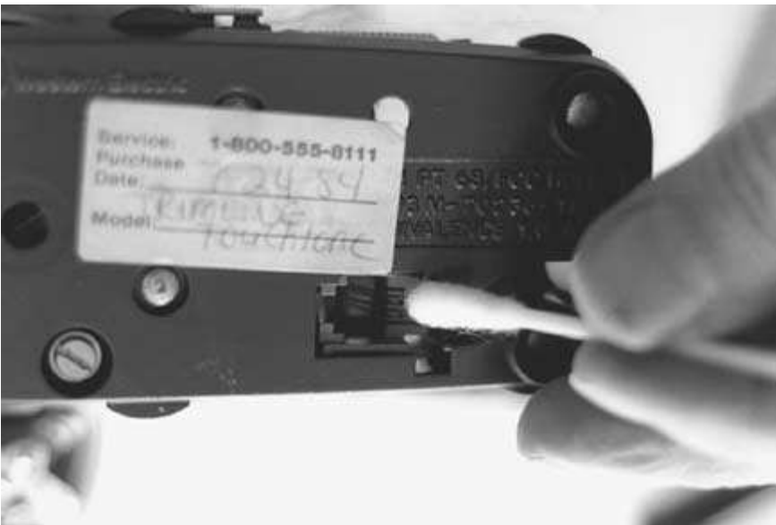
FIGURE 8-13 Clean the module jack with a good contact cleaner or with isopropyl alcohol.
