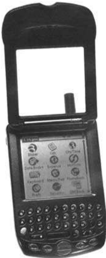
FIGURE 8-56 The Handspring Treo model 180 is a PDA smart phone with many features and a full keyboard.
