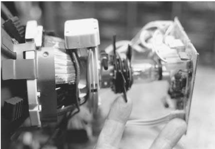
FIGURE 4-21 This photo shows the GE in-gun assembly and the adjustments used for convergence.
