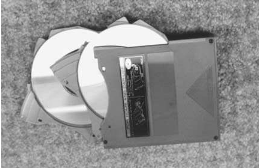
FIGURE 3-2 Another view of the Pioneer six-CD cartridge, showing how the discs swing out for replacement. This cartridge, when fully loaded, can provide approximately 6 hours of music.
