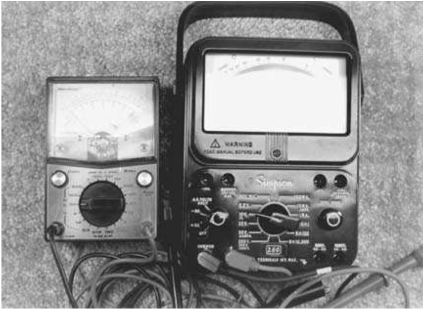
FIGURE 1-18 Volt/ohmmeters that can be used to check capacitors and other electronic components.
