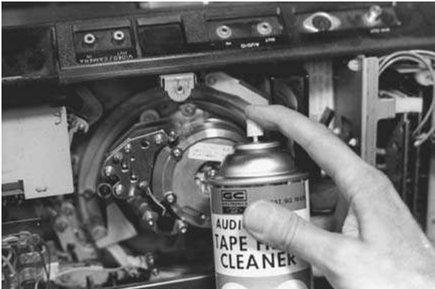
FIGURE 7-15 Audio/video head cleaner spray is being used to clean a camcorder's cylinder heads.
