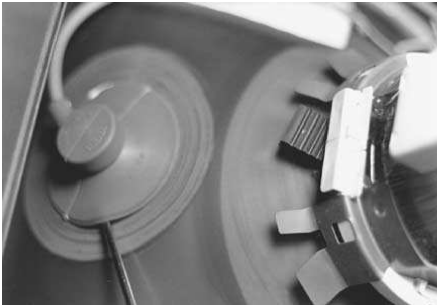
FIGURE 4-5 Location of the picture tube's high-voltage anode connection. Use caution when working around this section of a TV set or monitor.
