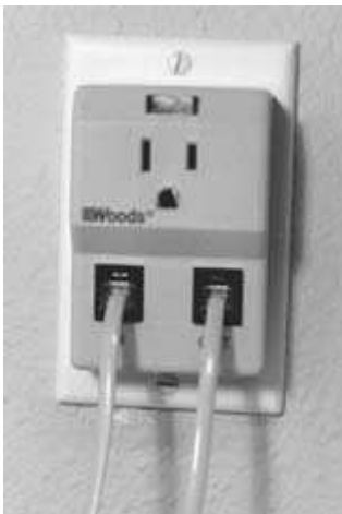
FIGURE 10-12 A surge-protection device for your printer that plugs into an ac outlet. It also has connections to plug in phone and fax equipment for phone-line protection.
