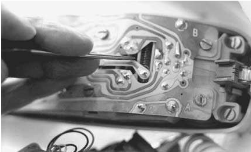
FIGURE 8-14 Location of the hook switch slide contacts.
