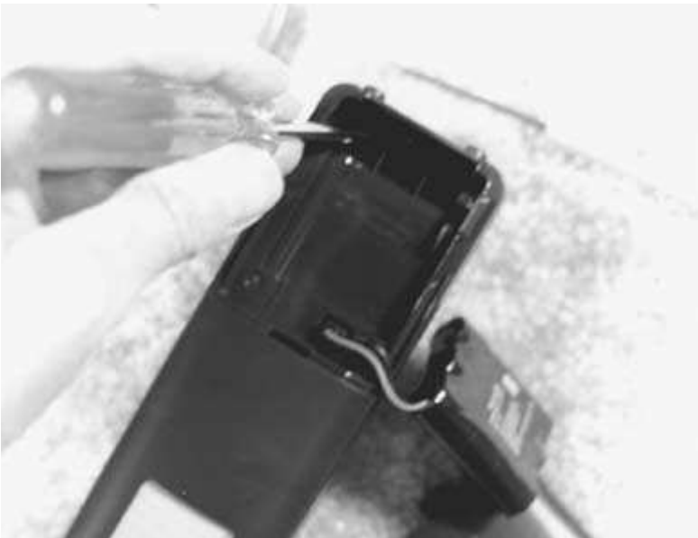
FIGURE 8-40 Take off the battery cover and remove the battery. Then take out the screws to separate the two handset covers.
