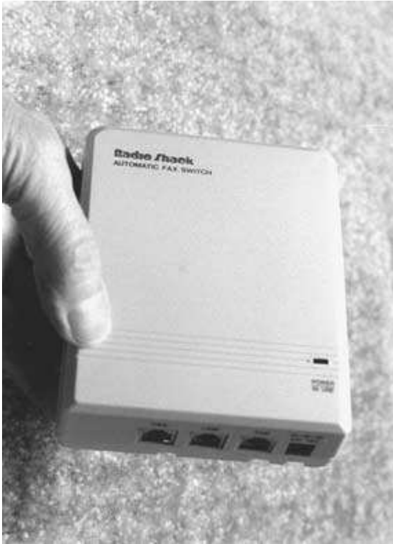
FIGURE 10-17 With this Radio Shack automatic fax machine switchover unit, you need only one phone line for voice phone and fax machine operation.
