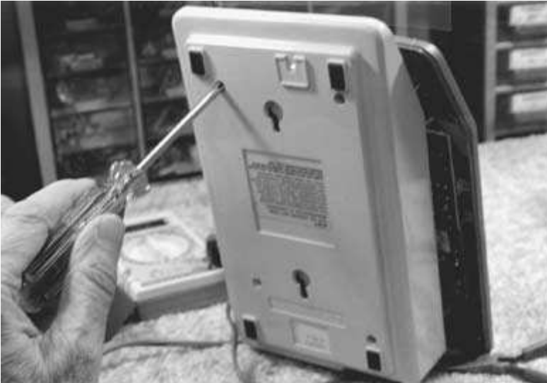
FIGURE 8-39 To repair or clean the phone, remove the four screws from the base unit.
