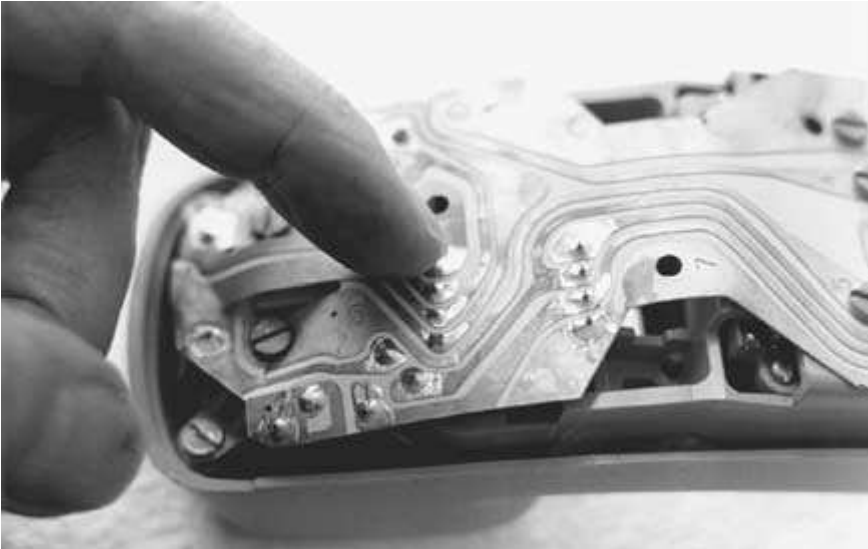
FIGURE 8-15 A poorly soldered connection might cause the phone to be dead or operate intermittently.
