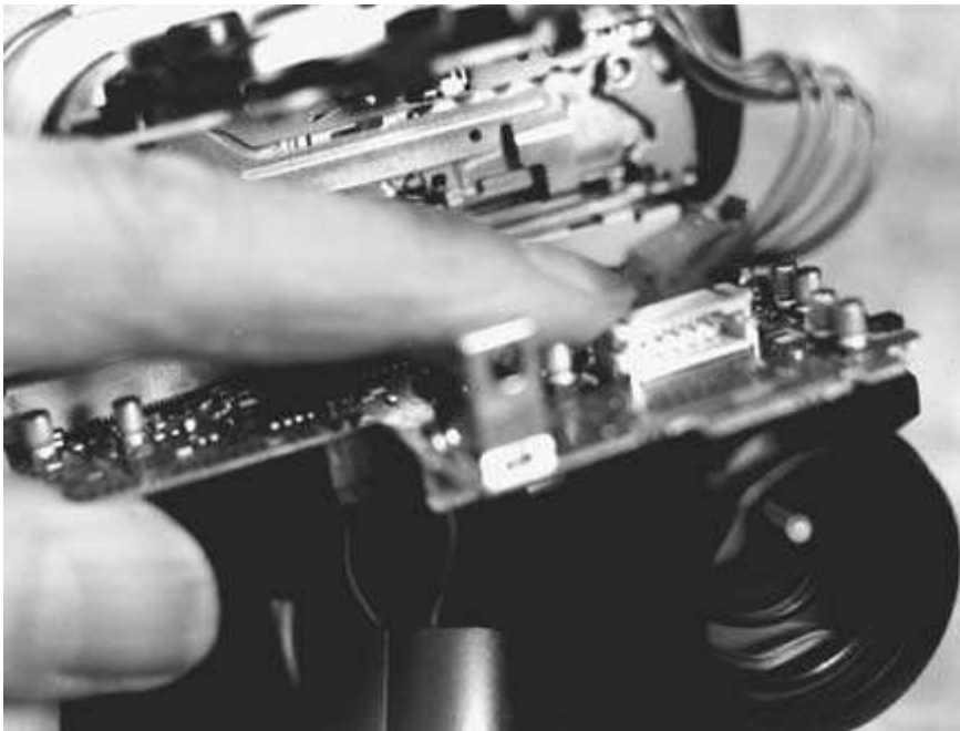
FIGURE 7-22 Inspect the zoom/focus circuit board for any poor connections and clean any flex cable connector contacts with isopropyl alcohol.
