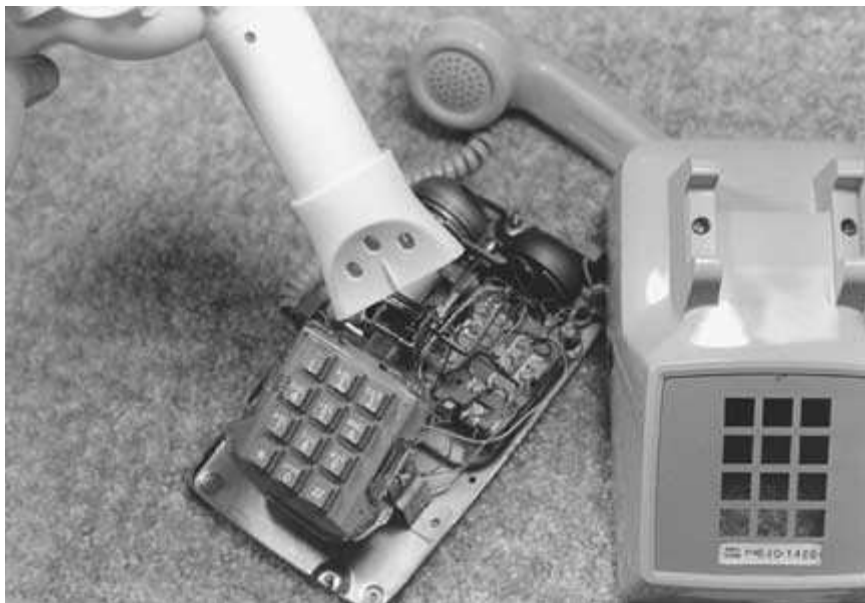
FIGURE 8-9 After flushing out the phone with clean water or an electrical contact cleaner, use a blow dryer to dry out the circuitry. This can be used for other types of electronic equipment also.
