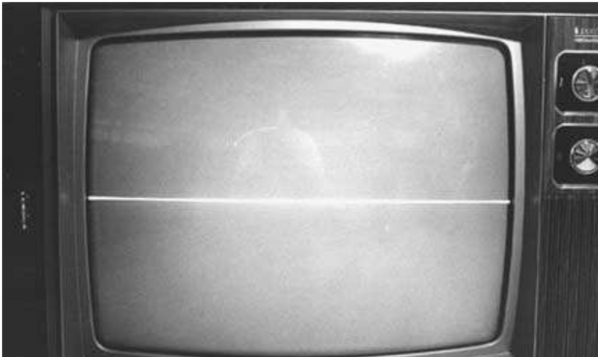
FIGURE 4-9 A thin, white horizontal line indicates a vertical sweep failure.
