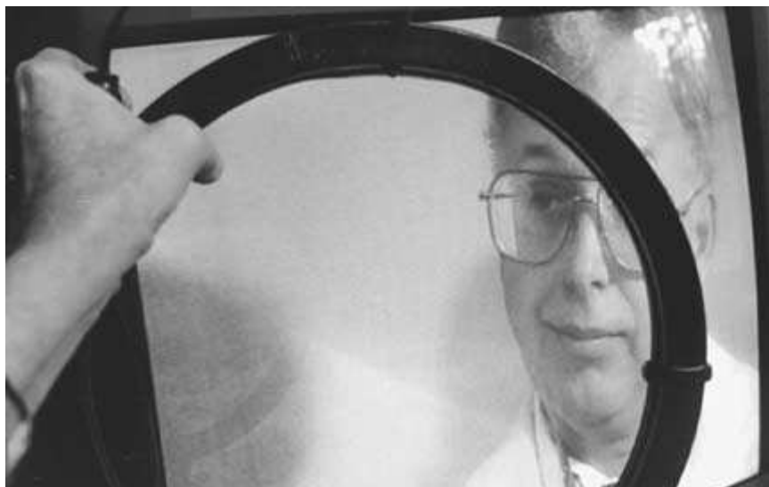
FIGURE 4-24 A degaussing coil being used to demagnetize a color TV picture tube faceplate.
