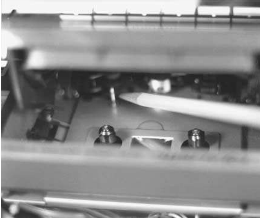
FIGURE 2-27 The tape can wrap around the capstan. Remove the tape and clean the spindle with alcohol.
