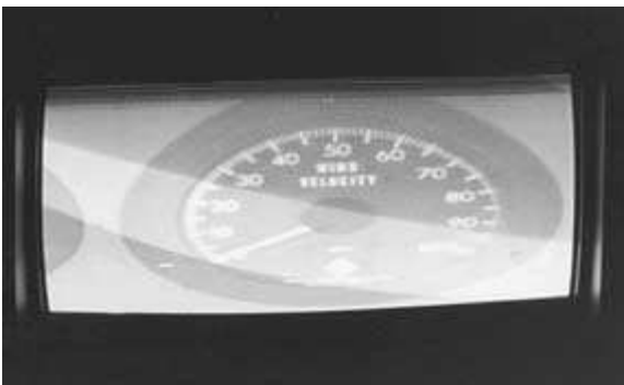
FIGURE 4-34 The picture pulled down from top and bottom. This is usually a vertical sweep circuit problem.
