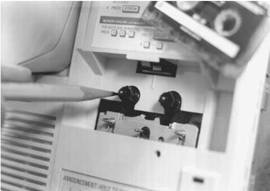
FIGURE 8-23 The hub gears turn the tape spools within the cassette unit.
