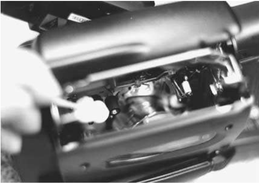
FIGURE 7-18 A sponge swab soaked in cleaning fluid is being used to clean the cylinder heads.
