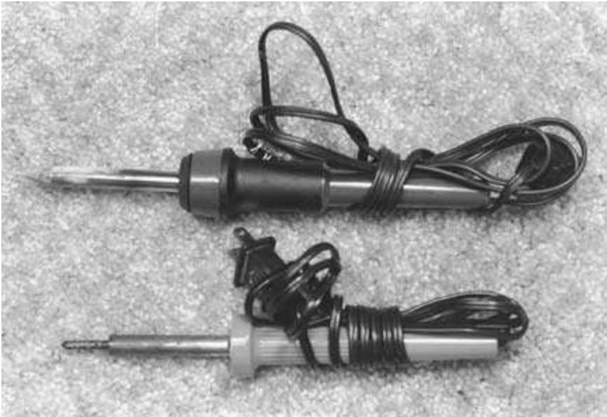
FIGURE 1-46 A 25-watt (bottom) and a 45-watt soldering iron.
