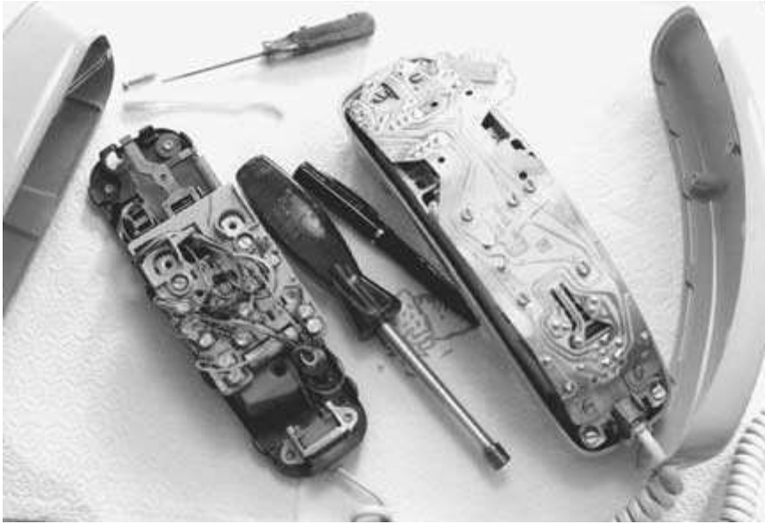
FIGURE 8-11 A Western Electric Princess phone taken apart for cleaning and repairs.
