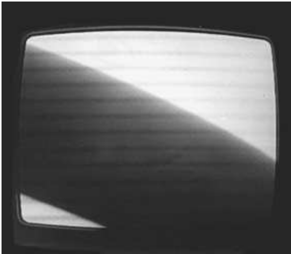
FIGURE 4-35 Small narrow black lines appear across the screen, and the picture might bend or weave.
