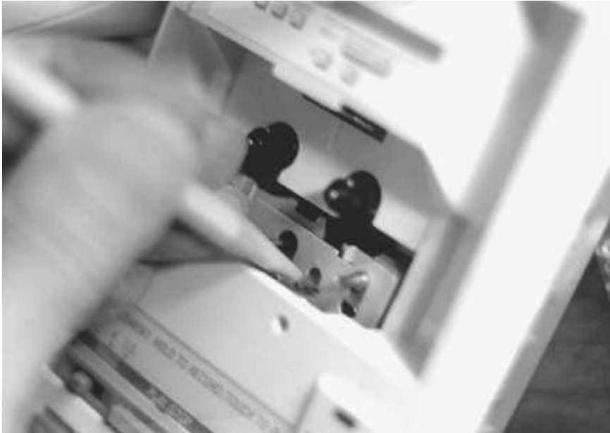
FIGURE 8-26 The record/play head can be cleaned without removing the top case of the answering machine.
