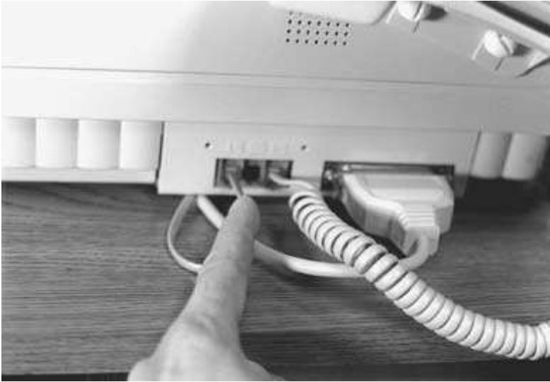
FIGURE 10-13 For intermittent fax problems, be sure all module phone plugs are clean and tightly connected.
