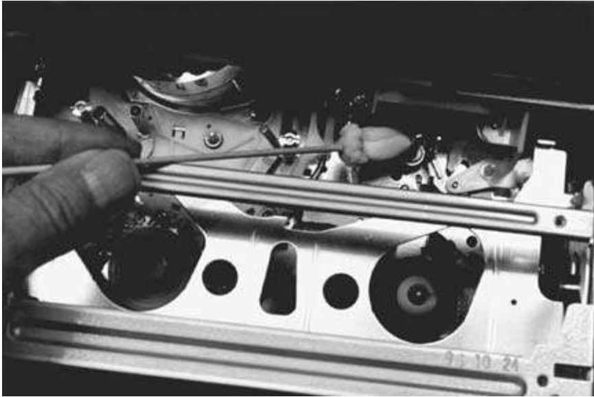
FIGURE 7-20 The various rubber rollers and tape path guides should also be cleaned when the tape head is being cleaned. You can use isopropyl alcohol for this process.
