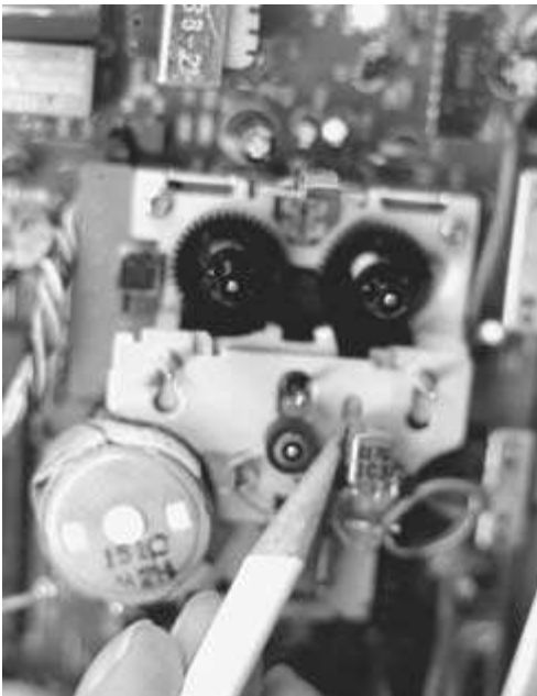
FIGURE 8-24 The capstan and pinch roller is to the left of the pencil pointer and the record/play head is on the right.
