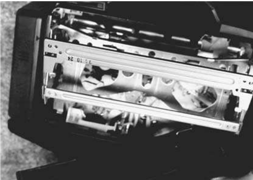
FIGURE 7-17 The camcorder tape door cover has been removed to make cleaning the heads and other parts easier.
