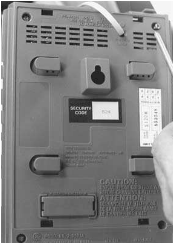
FIGURE 8-29 For cleaning and repair, remove four screws from bottom of the machine.
