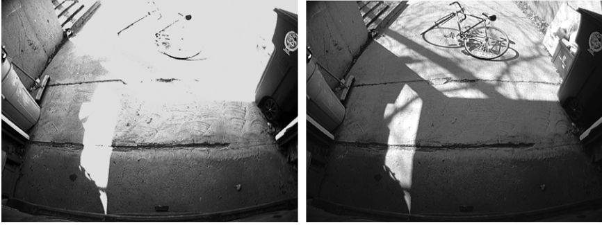
8.4 Side-by-side comparison of a linear image and a high dynamic range image. The linear image shows a saturated zone with resulting loss of information because the scene dynamic range is larger than the dynamic range of the camera.
