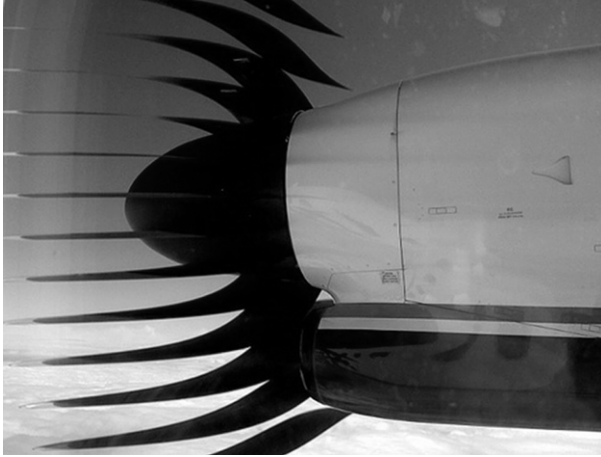
5.10 A scene showing the effects of rolling shutter on fast moving scenes.
