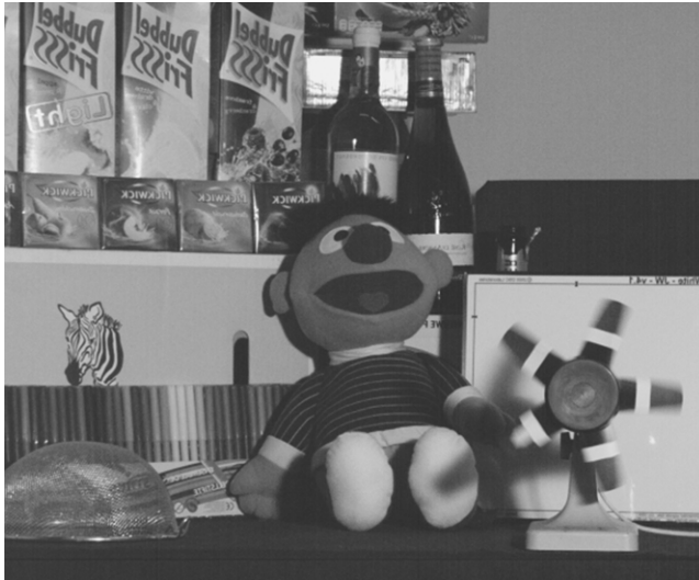
13.21 Image after DDS at 1920 × 1080p60 in global shutter mode at 1 ms integration time (Jeroen Rotte, Grass Valley, Nederland BV).
