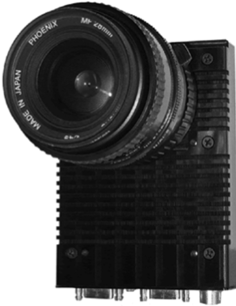
14.13 A super-lattice doped CMOS camera optimized in deep UV (260 nm) for wafer and reticle inspection applications.
