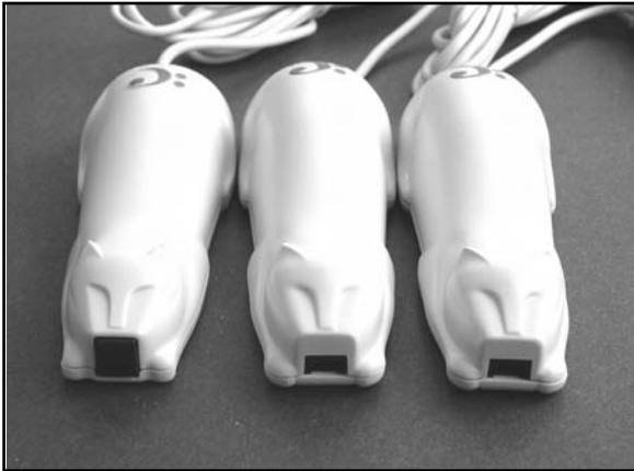
Figure 3.40 Front of CueCat Showing Scanning “Orifice” Variations: Left, Four-Screw PS/2; Center, Two-Screw PS/2; Right, USB
