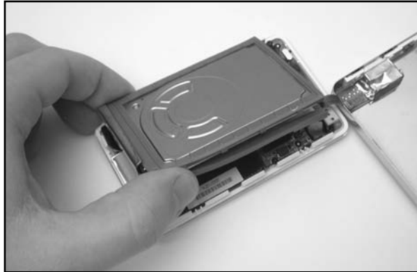
Figure 11.25 The Third-Generation iPod Opened and Ready for the Hack
