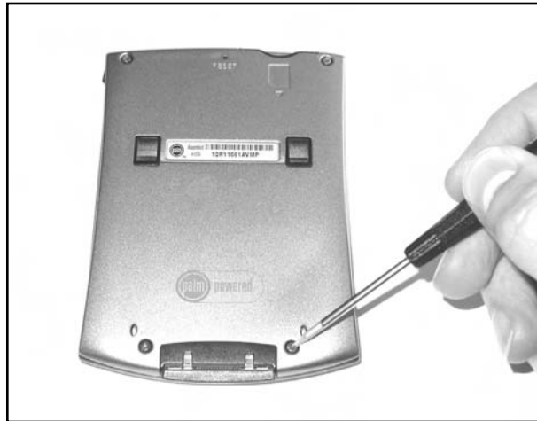
Figure 13.29 Unscrewing the Palm m505
