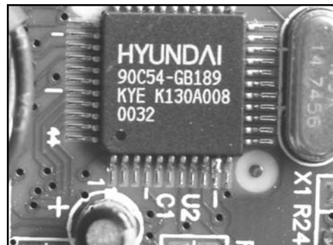
Figure 3.34 Hack Complete: Pin 10 of Microprocessor Lifted (Close-Up)
