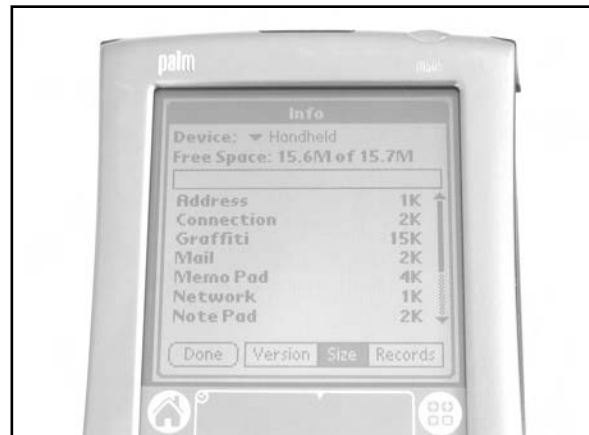
Figure 13.42 After Hack: Palm m505 With 16MB RAM
