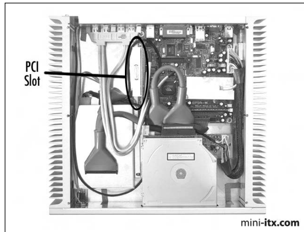
Figure 6.4 An Interior View of the Silent Mini-ITX PC Case (Photo Courtesy of Mini-itx.com)
