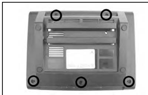
Figure 7.37 Remove Screws as Shown
