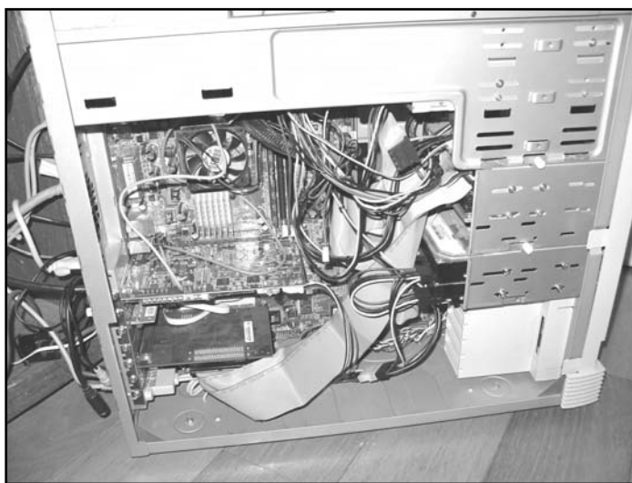
Figure 6.5 Interior of the Windows HTPC System
