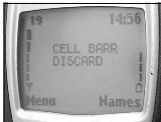
Figure 12.31 Test 19: Ignoring Barred Base Stations
