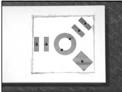
Figure 4.13 Template With Pilot Holes and Initial Cuts
