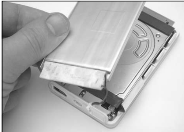
Figure 11.19 Removing the Old Battery
