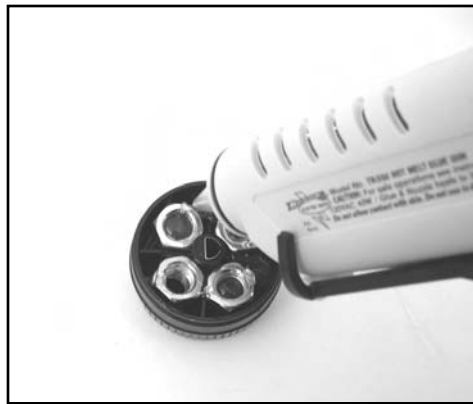
Figure 8.34 Gluing the Nuts in Place
