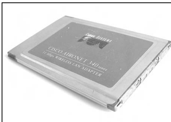
Figure 10.2 A Cisco Card with Dual MMCX Connectors
