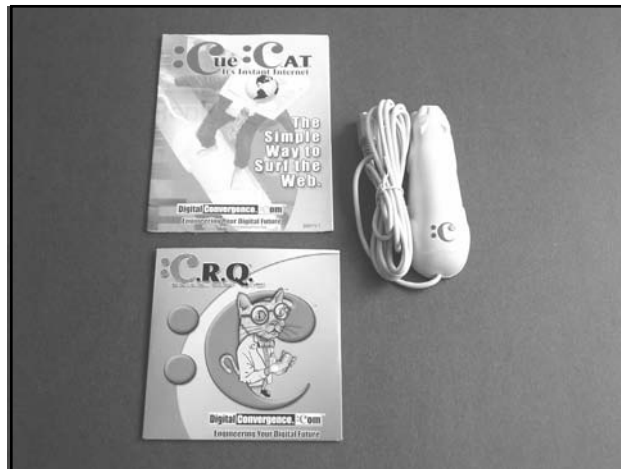
Figure 3.1 The CueCat Optical Reader, Four-Screw PS/2 Interface with Original Materials
