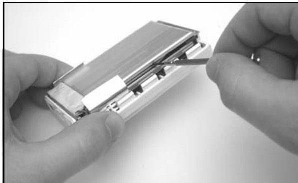
Figure 11.18 Prying the Battery from the Rubber Strips
