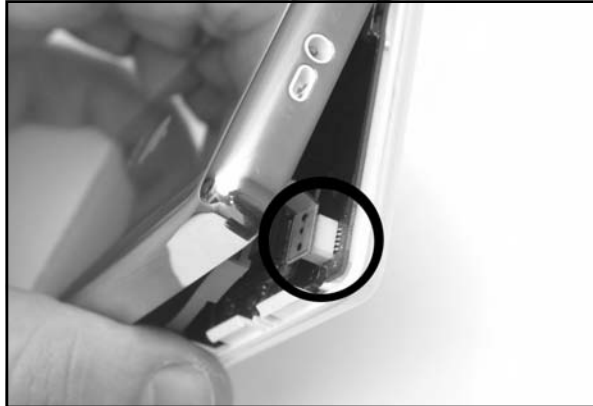
Figure 11.14 Connector Holding Two Halves Together
