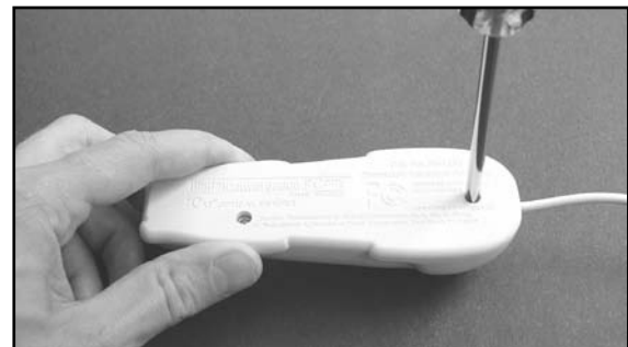
Figure 3.9 Unscrewing the CueCat
