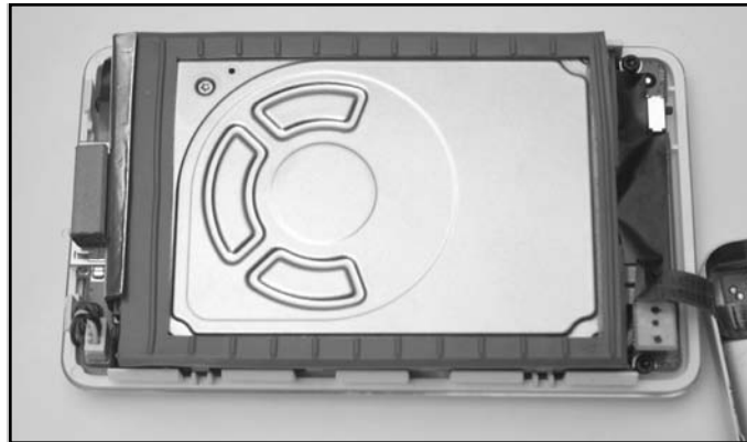
Figure 11.34 Hard Drive Back in Place
