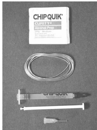
Figure 2.33 ChipQuik SMD Removal Kit Contents
