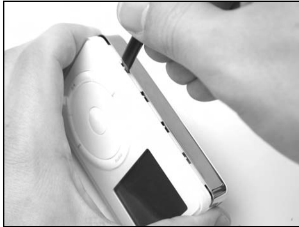
Figure 11.8 Continue Working Down the Edge
