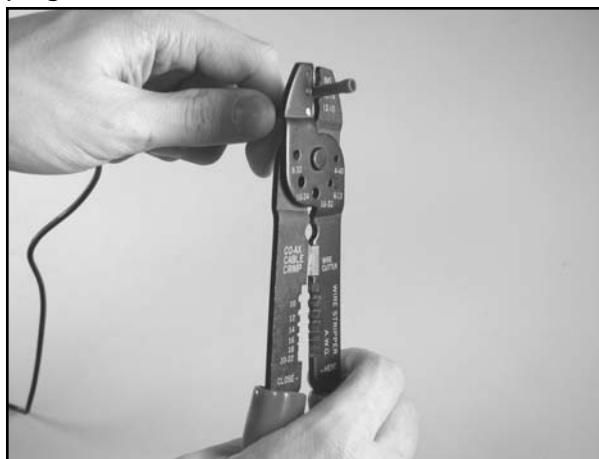
Figure 5.47 Crimping the Wire
