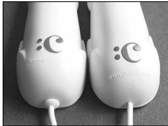
Figure 3.41 Back of CueCat Showing Connector Cable Variations: Left, Four-Screw PS/2; Right, Two-Screw PS/2
