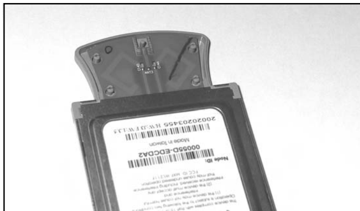
Figure 10.7 Inside the Antenna Compartment
