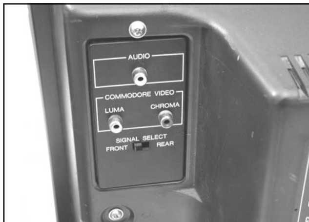
Figure 8.71 Commodore 1702 Rear Input Jacks
