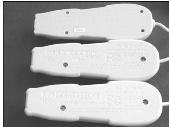
Figure 3.3 Bottom of the CueCat: Top, Four-Screw PS/2; Middle, Two-Screw PS/2; Bottom: USB
