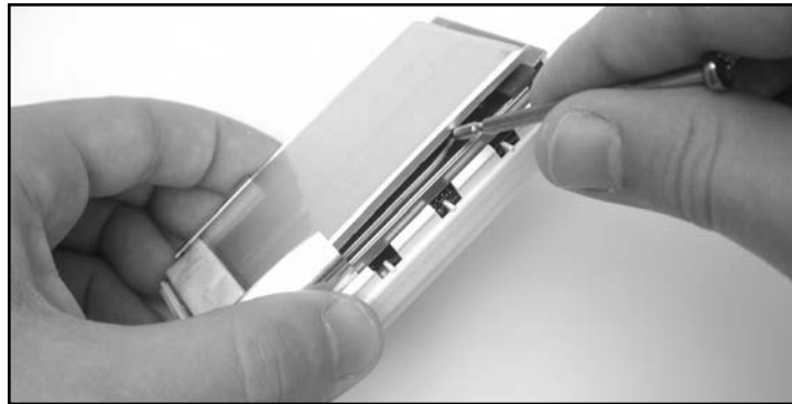
Figure 11.40 Pulling the Battery and Hard Drive Apart
