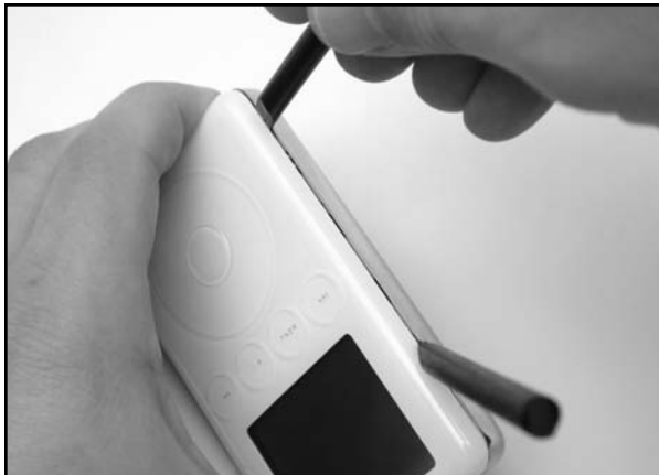
Figure 11.11 Continue Prying Along One Side
