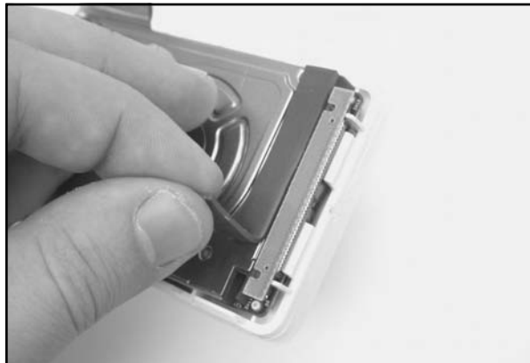
Figure 11.42 Removing the Rubber Pads
