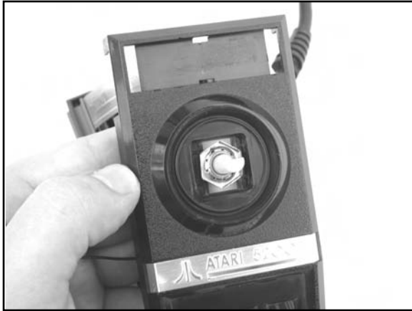
Figure 8.29 Assembling the 2600 Potentiometer
