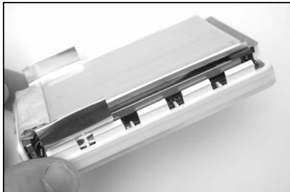
Figure 11.52 Battery Back in Place
