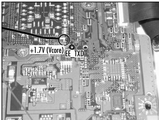
Figure 9.11 The V CORE , EE_TXD, and EE_RXD
