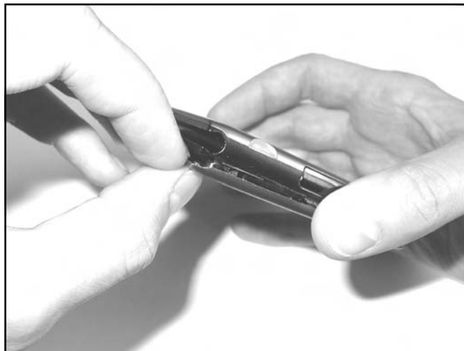
Figure 13.30 Removing the Metal Backing
