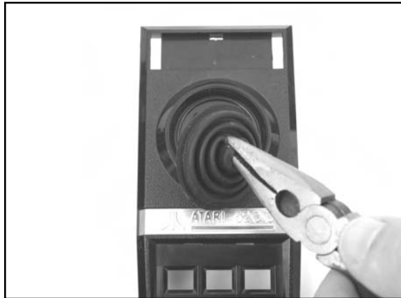
Figure 8.28 Removing the Rubber Joystick Boot
