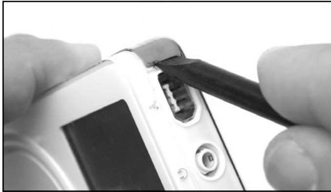
Figure 11.6 Start Prying at the Top of the Case
