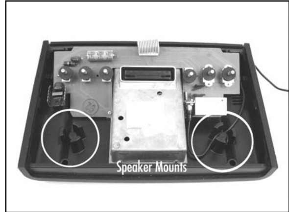
Figure 7.23 Receptacles Inside the Case for Speakers
