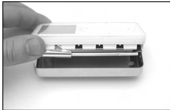
Figure 11.9 Lifting Apart the Two Halves of the iPod
