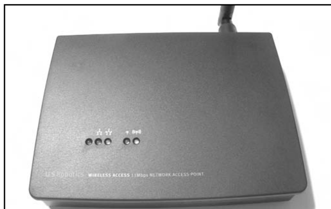
Figure 10.13 The USR 2450 Access Point before Modification
