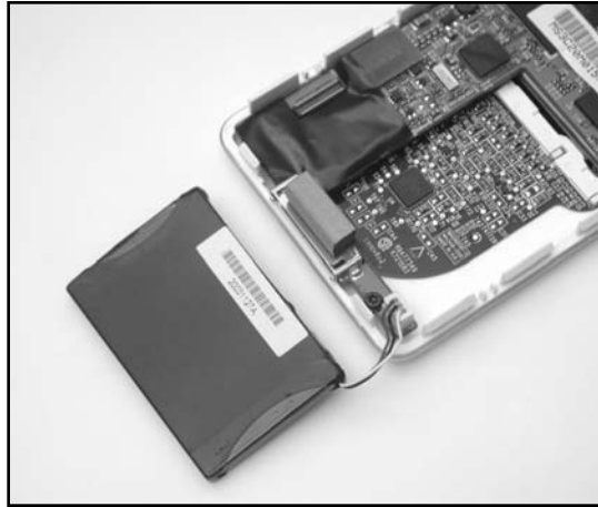
Figure 11.29 The iPod Battery Removed
