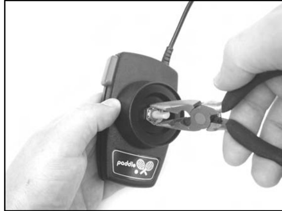
Figure 8.17 Removing the Paddle Nut
