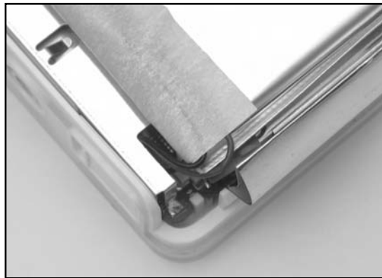
Figure 11.22 Power Cable Safely Tucked Away
