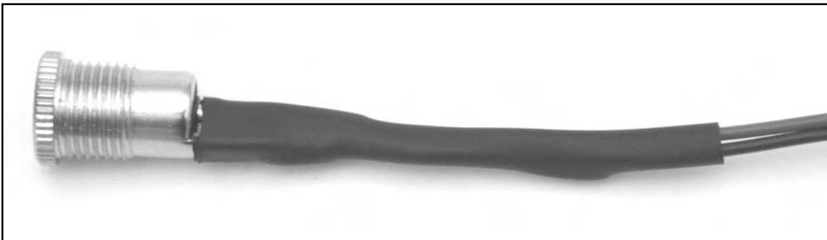
Figure 8.44 Building the Power Cable
