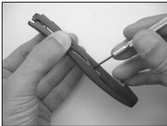
Figure 12.6 Step 2: Releasing the Plastic Housing Clips from the Other Side of the Phone
