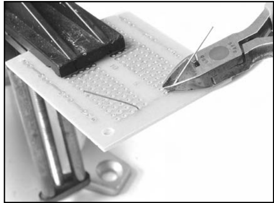
Figure 2.31 Snipping Off the Remaining Component Lead
