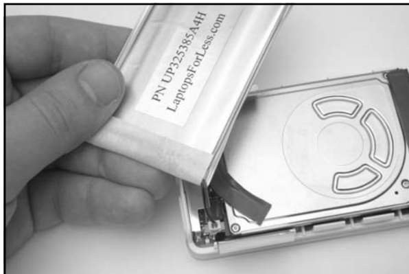
Figure 11.20 Connecting the New Battery
