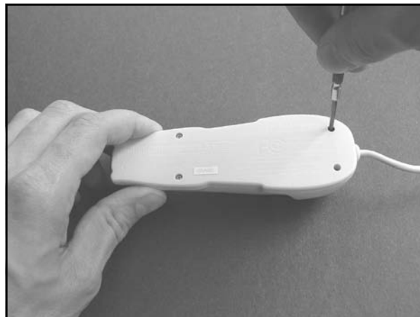
Figure 3.4 Unscrewing the CueCat
