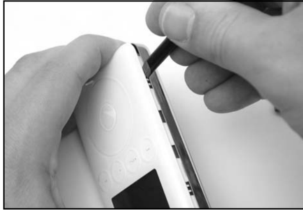
Figure 11.12 Unclip all the Tabs
