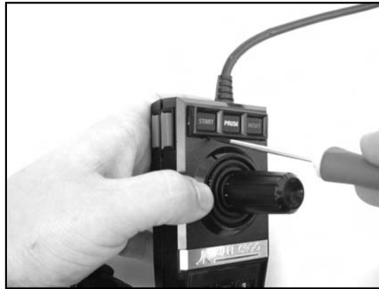
Figure 8.21 Removing the Upper Bezel
