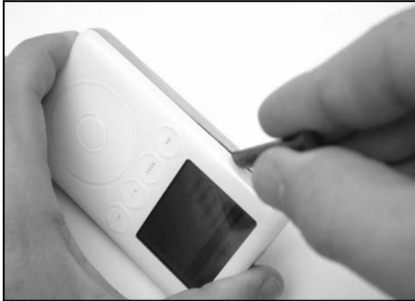
Figure 11.10 Prying into the Case
