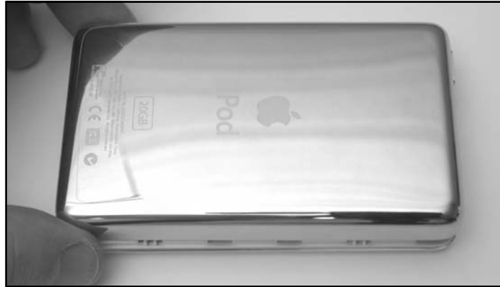
Figure 11.35 Snapping the Case Back Together
