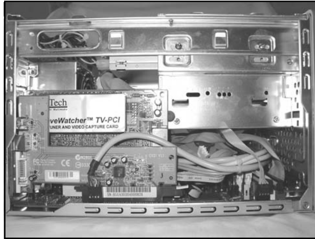
Figure 6.31 The Two Cards Installed in the Shuttle Case
