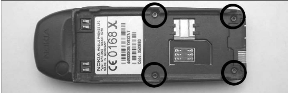
Figure 12.4 The Back of the Nokia 6210 with Battery Removed; the Four Torx Screws Are Visible
