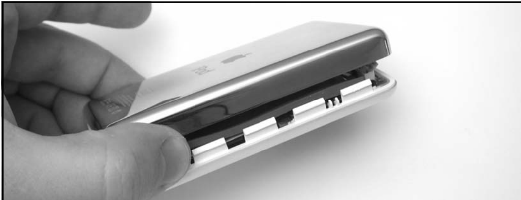
Figure 11.13 Opening the Case
