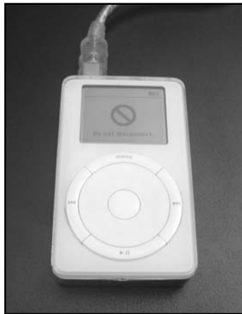
Figure 11.24 Charging the New Battery
