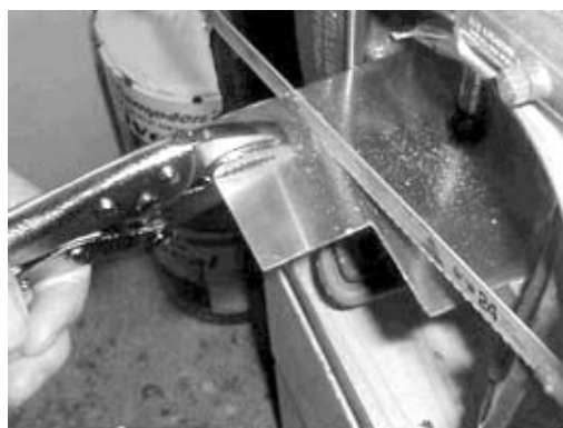
Figure 4-5. Bend the metal sheet
