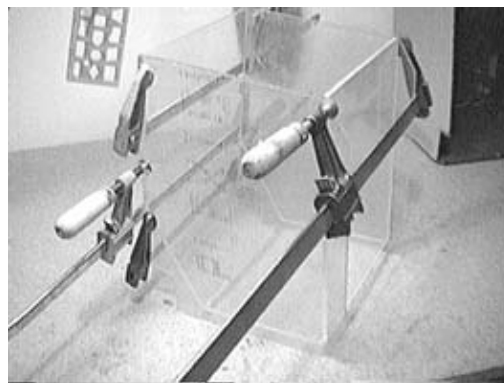
Figure 2-55. Apply solvent for seal to bottom
