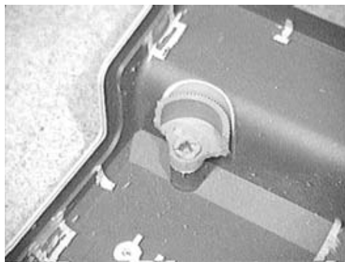
Figure 2-66. Cut away brightness knob material
