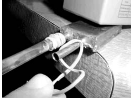
Figure 4-19. Rubber band hose clamps
