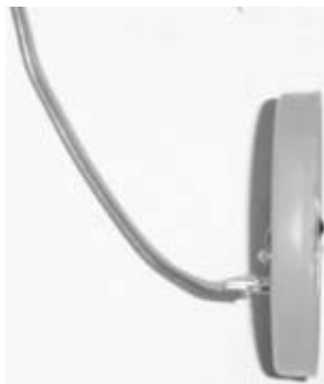
Figure 13-4. IR receiver mount side view
