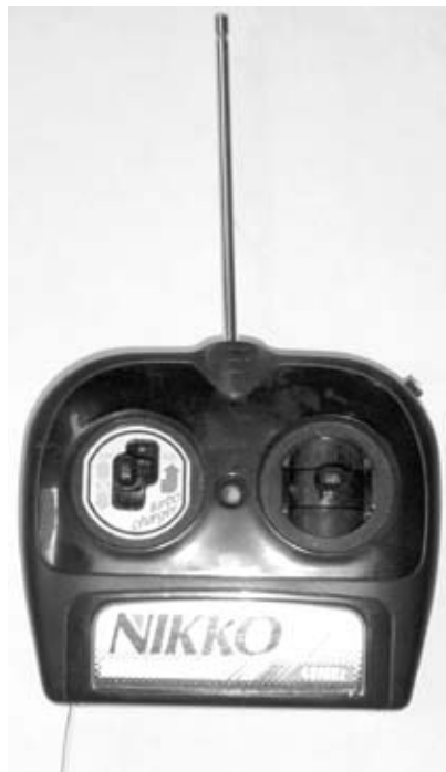
Figure 13-10. Completed controller with trigger transmission
