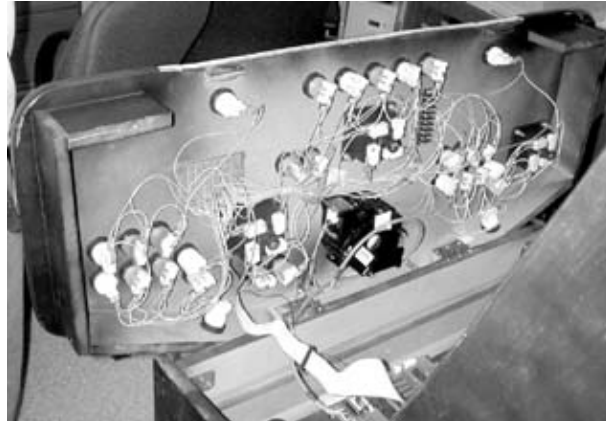
Figure 11-12. Completed button wiring
