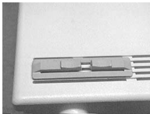
Figure 2-68. Replaced programmer's switch
