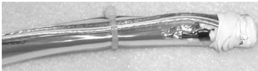
Figure 15-12. Temperature and water sensor final sealing
