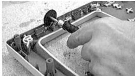
Figure 2-22. Front case plastic removal
