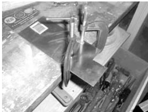
Figure 4-3. Secure the metal sheet
