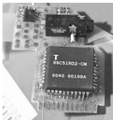
Figure 5-22. Main processor in place
