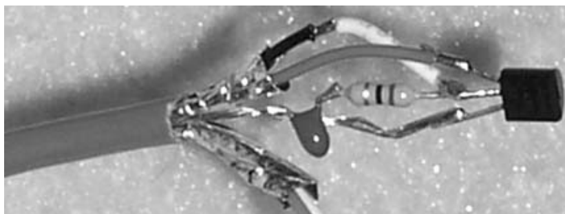
Figure 15-8. Temperature sensor wiring
