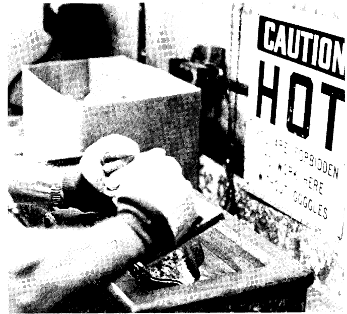
FIG. 7.6 Slush casting pattern being dipped in melt pot. (Reproduced through the courtesy of Cerro Metal Products Corp.)
