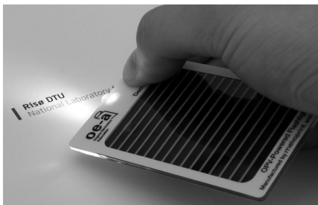
17.18 Credit card sized lamp with built in organic solar cell, lithium ion battery, diodes and LED. Danish research institute Risø DTU (now DTU Energy Conversion) and Mekoprint built the demonstrator in more than 10 000 units.
