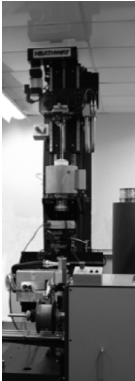
25.5 Fiber draw tower for polymer optical fiber.
