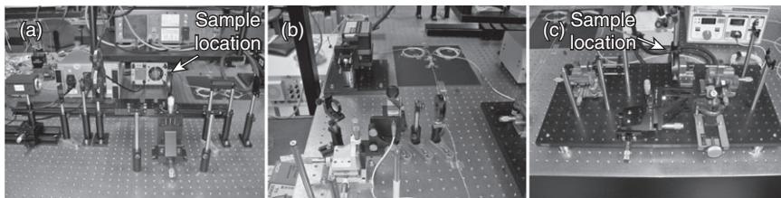
25.34 Pictures of characterization setup for SLM: (a) portion of setup for measuring image throughput of SLM; (b) portion of setup for coupling lasers and broadband source; (c) portion of setup for performing individual pixel characterization.
