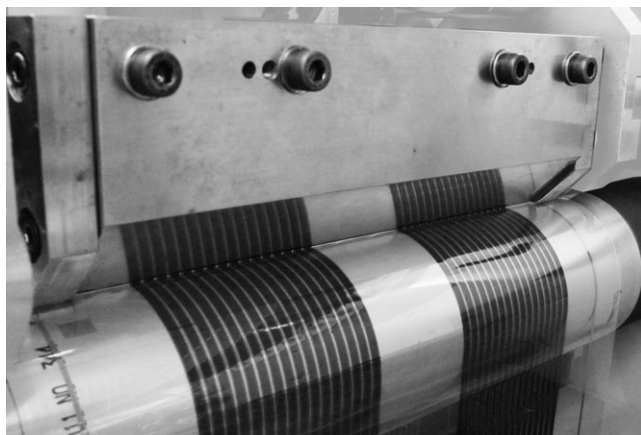
17.10 Slot-die coating of P3HT:PCBM solution for the active layer of OSCs. 32 stripes of 5 mm width are coated parallel. The gap between each stripe is 1 mm.
