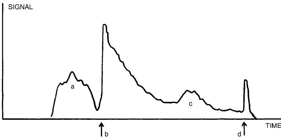
Figure C3.2.42. Schematic of water and seabed scattered return signals: (a) haze or “sea smoke”; (b) surface return; (c) scattering layer; (d) seabed return.
