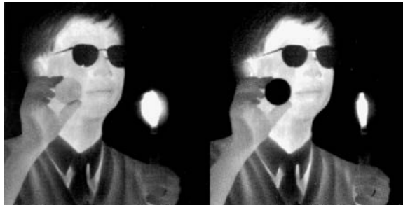
Figure A1.4.47. Simultaneous images from 256 × 256 MWIR/LWIR QWIP FPAs. Note appearance of the front-held filter and the hot soldering iron in the two bands. Reproduced from [28].
