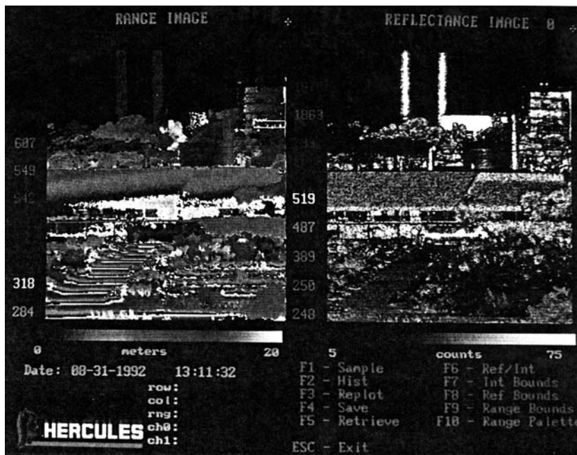
Figure C3.2.35. Range and reflectance imagery with a 1.047\ \mu\text{m} direct detection lidar at 2 km, collected with the Hercules Corporation system (from Ref. [192]). Much detail is lost in transcription from the original false colour imagery.
