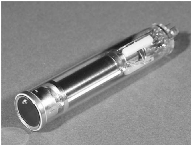
Figure C2.1.11. Appearance of the ultrahigh sensitivity HARP camera tube.
