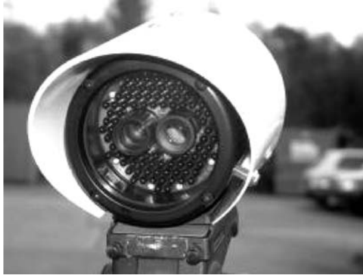
Figure C4.2.2. P362 camera with integral illuminator and overview camera. (Courtesy of PIPS Technology Ltd.)
