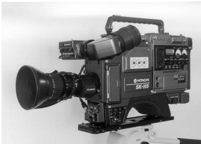
Figure C2.1.14. Appearance of the ultrahigh sensitivity HARP colour camera.
