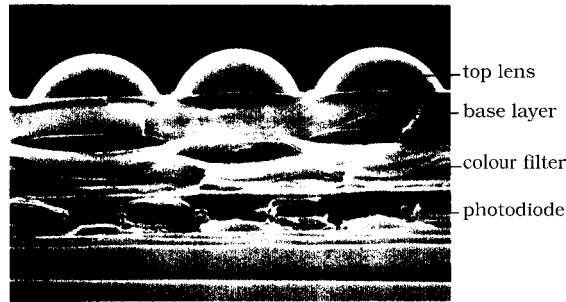
Figure C2.1.28. Cross-sectional view of micro-lens structure. (Photograph courtesy of H Komobuchi, Matsushita Elect. Co.)
