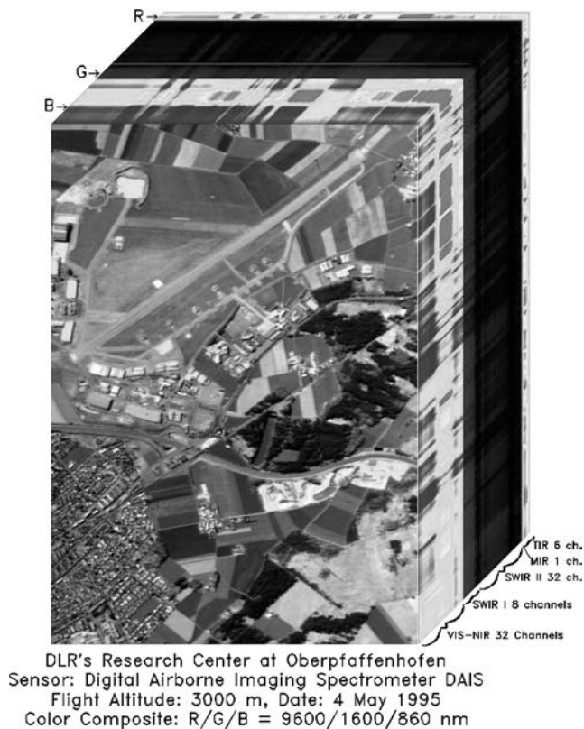
Figure B8.29. Colour composite image recorded using the Digital Airborne Imaging Spectroradiometer (DAIS) (with permission from German Aerospace Center DLR) (see http://www.op.dlr.de/dais/dais-gal.htm ).
