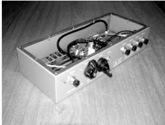
Figure C4.2.5. P367 video recognizer for roadside deployment. (Courtesy of PIPS Technology Ltd.)
