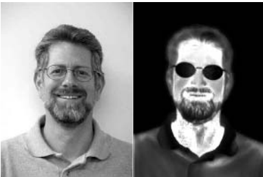
Fig. 3.47. Photographs in visible light and infrared thermal radiation which is naturally emanated from the object. Note the brighter (appearing warmer) areas at the wrinkles and skin folds near the nose—a result of the cavity effect. Eyeglasses appear black (cold) because glass is opaque in the mid- and far-infrared spectral ranges and does not pass thermal radiation from the face. (Photo courtesy of Infrared Training Center, www.infraredtraining.com .)
