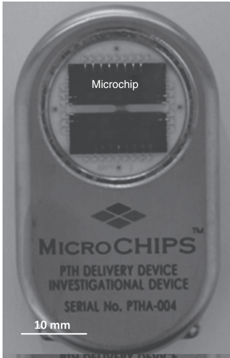
15.4 The MicroCHIPS® micro-reservoir device (Farra et al. , 2012, reprinted with permission from AAAS).
