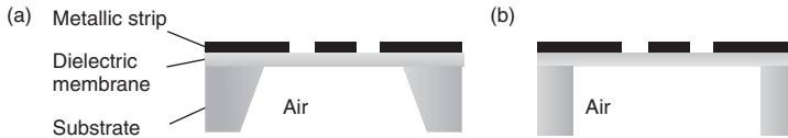
3.1 Illustration of bulk micromachined coplanar lines obtained with (a) wet and (b) dry etching techniques.
