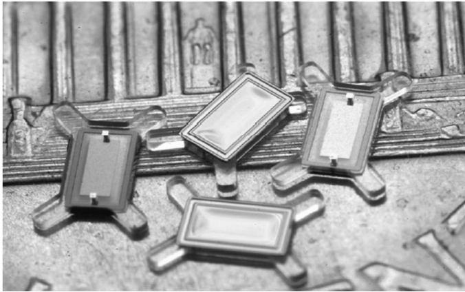
14.15 Capacitive pressure sensors made from a glass reflow process in silicon upon a U.S. penny (reproduced with permission from Wise, 2010).
