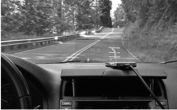
18.15 Direct projection see-through Auto-HUD using a surface with narrowband reflectance corresponding to a picoprojector's laser light sources.
