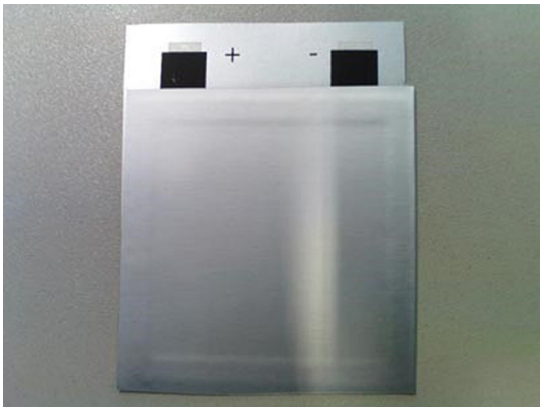
Figure 18.7 Cell after folding with both contacts on the same side of substrate.
