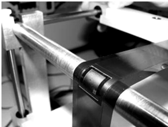
Figure 6.14 Foil-based thin-film battery ( 10 \times 10 mm 2 ) bent to 6.5 mm bending radius. Source: Ref. Seventh Framework Programme .
