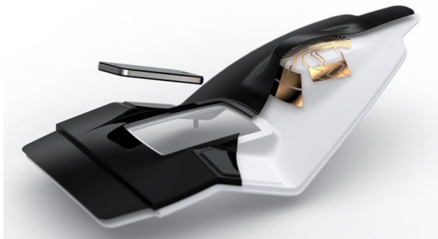
Figure 14.7 Touch-sensitive intelligent surface that replaces mechanical switches, sliders and wheels with capacitive electronics.
