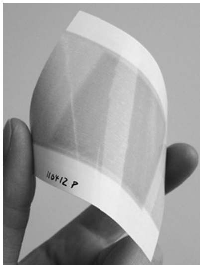
Figure 7.24 Photograph of printed paper loudspeaker demonstrating its flexibility. Reproduced from Hübler et al. (2012) with permission from Elsevier.
