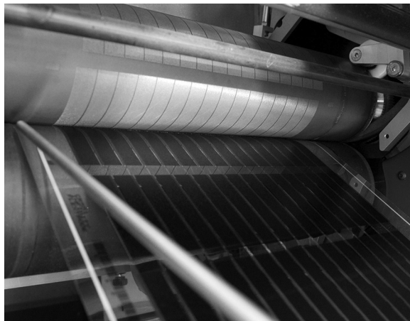
Figure 7.4 Rotary screen-printing of PEDOT:PSS, the printing pattern is visible on the screen (top of the picture).
