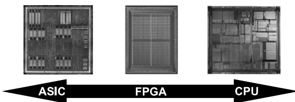
Fig. A.1 On a continuum of generality, CPUs are the most programmable, and ASICs are the least
