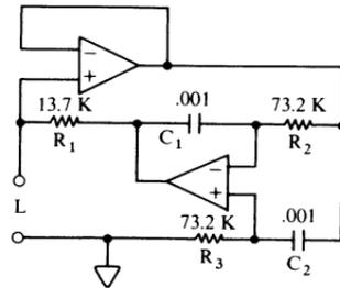
With only a high Q capacitor connected to the L input and  $R_3$  tweaked to the edge of oscillation, circuit Q is very close to infinite.
