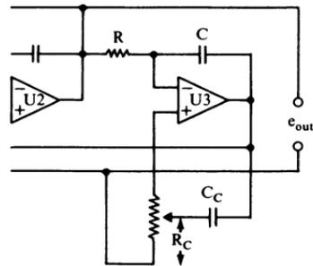
Short  $R_0$  and tweak  $R_c$  or  $C_c$  to the edge of oscillation for best general formula accuracy. This also compensates for capacitor  $Q$ .
