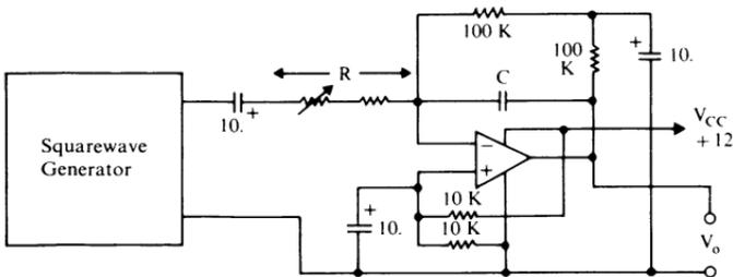
$$V_{op-p} = (V_{in})_{p-p}/(2fRC)$$
