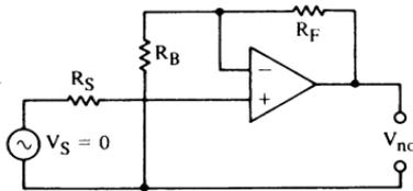
$$V_{no} = A_v \sqrt{BW} \sqrt{V_n^2 + I_n^2 (R_S + R_X)^2 + 4k_B T_K R_S}$$
