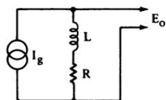
**Note:**  $\text{---}\text{---}$  = Infinite impedance alternating current source
