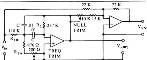
$$|A_{VO}|_N = -40 \text{ dB}, \quad BW_{N(-40 \text{ dB})} < 1 \text{ Hz}$$
