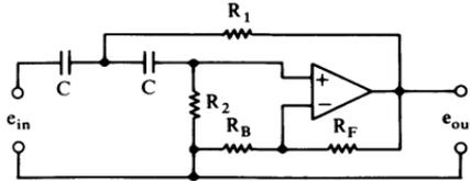
$$|A_{v\text{hf}}| = 1 + R_F/R_B, \quad |A_{v\text{fo}}| = (1 + R_F/R_B)/d$$
