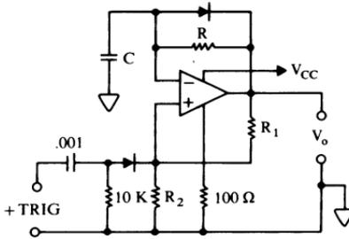
$$t_{on} = -RC(\ln[1 - (R_1/R_2 + 1)^{-1}])$$
