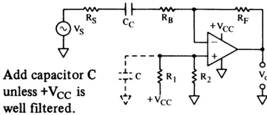
$$V_{O(DC)} = V_{CC}/2 \quad \text{when } R_1 = R_2$$
