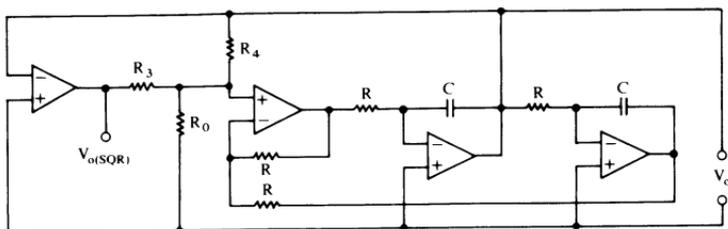
$$f_0 = [2\pi RC]^{-1}, \quad Q = (1 + R_4/R_3 + R_4/R_0)/2$$
