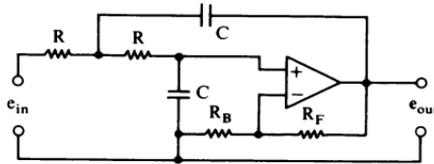
$$|A_{vlf}| = 1 + R_F/R_B, \quad |A_{vfo}| = (1 + R_F/R_B)/d,$$
