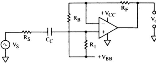
$$V_{O(DC)} = +V_{BB} \pm V_{OO} \quad \text{See } -V_{OO}$$
