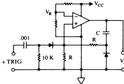
$$t_{on} = 2RC(\ln[V_{o(MAX)}/2V_R])$$
