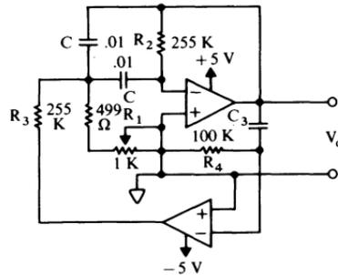
$$f_0 = [2\pi C\sqrt{R_1 R_2}]^{-1} \approx 850 \text{ to } 1350 \text{ Hz}$$
