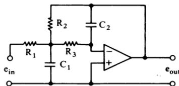
$$|A_{v|f}| = R_2/R_1, \quad |A_{v|fo}| = (R_2/R_1)/d$$
