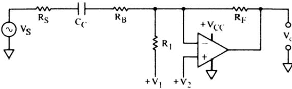
$$V_{O(DC)} = (V_2 [(R_F/R_1) + 1]) - [V_1 (R_F/R_1) \pm V_{OO}]$$
