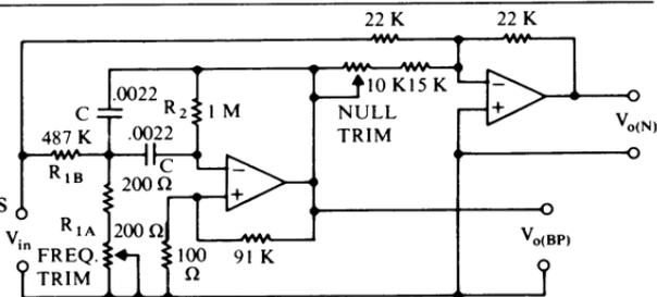
$$|A_V|_{\text{NOTCH}} < -40 \text{ dB}, \quad BW_{N(-40 \text{ dB})} < 1 \text{ Hz}$$
