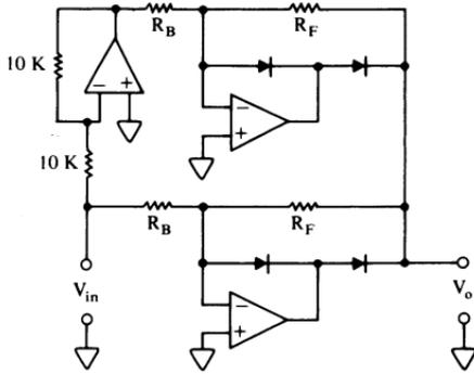
$$(V_o)_{pk} = (V_{in})_{p-p} R_F / 2R_B$$
