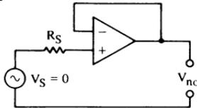
$$V_{no} = 100 \sqrt{V_n^2 + I_n^2 R_S^2 + 1.656 \cdot 10^{-20} R_S}$$
