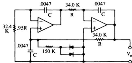
$$V_o \approx 2V_{p-p} \text{ (Very sensitive to tolerances)}$$
