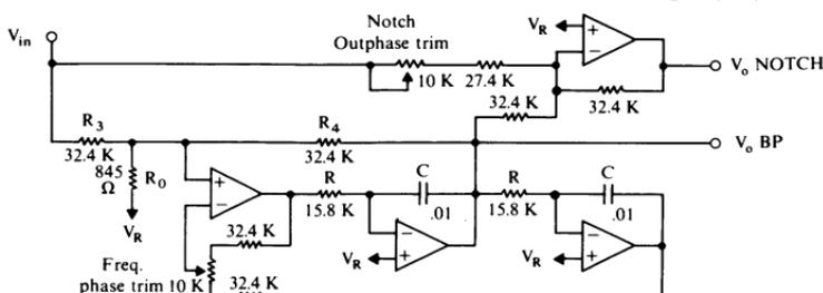
$$|A_V|_{\text{NOTCH}} < -40 \text{ dB}, \quad (BW_N)_{-40 \text{ dB}} < .5 \text{ Hz}$$
