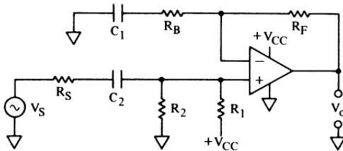
$$V_{O(DC)} = V_{CC}/2 \quad \text{when } R_1 = R_2$$
