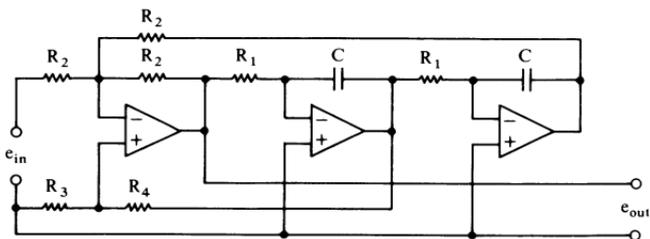
$$|A_{\text{vhf}}| = H_{\text{OHP}} = d^{-1} = (R_4/R_3 + 1)/3$$
