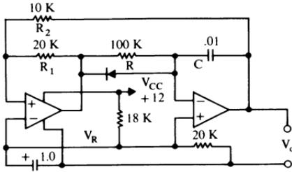
When  $R_1 > R_2$  and  $V_R = [(V_{SAT})_H + (V_{SAT})_L]/2$ :
