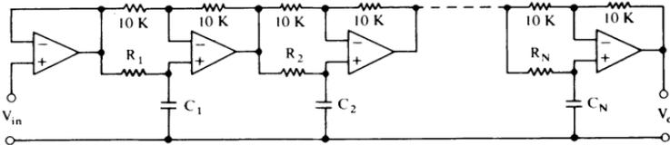
$$(\theta_e)_{out} = 2[\tan^{-1} (2\pi fR_1C_1)^{-1}] + 2[\tan^{-1} (2\pi fR_2C_2)^{-1}] \\ \dots + 2[\tan^{-1} (2\pi fR_NC_N)^{-1}]$$
