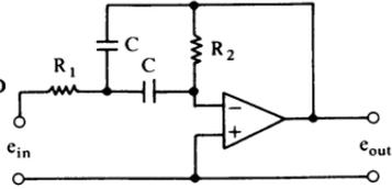
$$|e_{out}/e_{in}|_{dB} = 20 \log [R_2 / (2R_1 \sqrt{1 + Q^2 [(f/f_0) - (f_0/f)]^2})]$$
