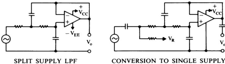
All general purpose opamp inputs must have dc continuity to a dc voltage source, to ground or to an opamp output.
