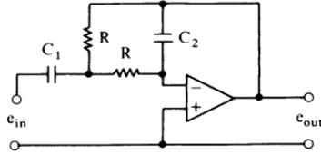
$$|e_{out}/e_{in}|_{dB} = 20 \log [2Q^2/\sqrt{1 + Q^2[(f/f_0) - (f_0/f)]^2}]$$
