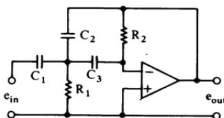
$$f_0 = [2\pi\sqrt{R_1 R_2 C_2 C_3}]^{-1}$$
