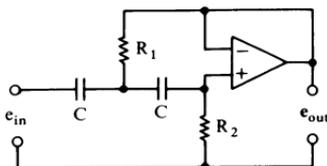
$$|A_{v_{hf}}| = 1, \quad |A_{v_{fo}}| = d^{-1}$$
