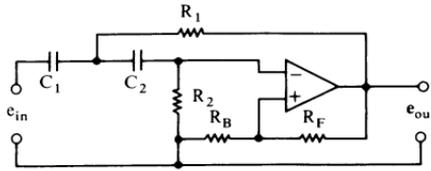
$$|A_{vhf}| = 1 + R_F/R_B, \quad |A_{vfo}| = (1 + R_F/R_B)/d$$
