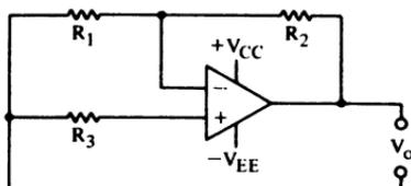
**Output from input offset voltage ( $V_{IO}$ ) only
