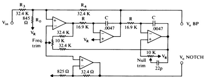
$$|A_{V0}|_{\text{NOTCH}} < -40 \text{ dB}, \quad \text{Notch BW}_{-40 \text{ dB}} < 1 \text{ Hz}$$
