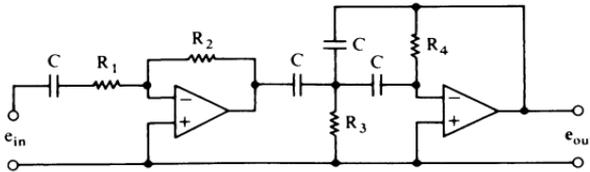
$$|A_V|_{\text{vhf}} = R_2/R_1$$
