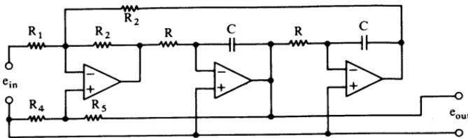
$$A_{VO} = H_{OBP} = QR_2/R_1 = (R_5/R_4 + 1)/(2R_1/R_2 + 1)$$
