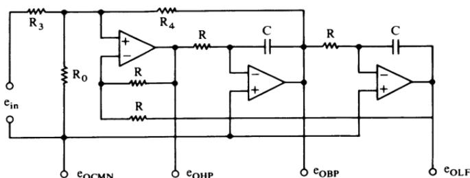
$$f_{\text{OHP}} = f_{\text{OBP}} = f_{\text{OLP}} = [2\pi RC]^{-1}$$
