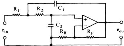
$$|A_{vlf}| = 1 + R_F/R_B, \quad |A_{vfo}| = (1 + R_F/R_B)/d,$$
