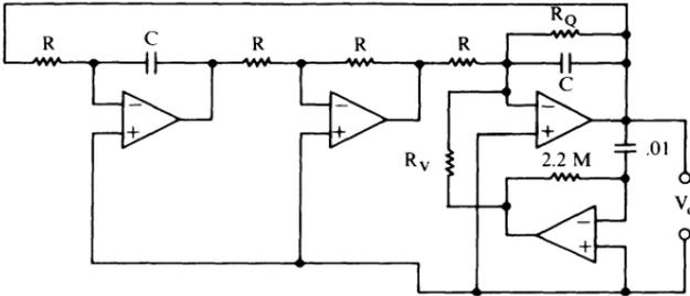
$$f_0 = [2\pi RC]^{-1}, \quad Q = R_Q(2\pi f_0 C)$$
