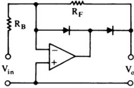
$$(V_o)_{pk} = (V_{in})_{p-p} R_F / 2R_B$$
