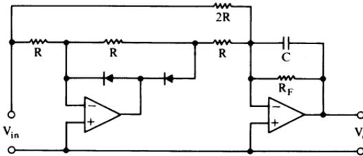
$$(V_o)_{dc} = (V_{in})_{av} R_F / 4R$$
