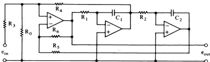
$$|A_{\text{vhf}}| = H_{\text{OHP}} = (1 + R_6/R_5)/(1 + R_3/R_0 + R_3/R_4)$$
