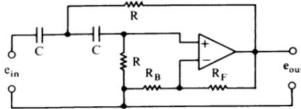
$$|A_{\text{vhf}}| = 1 + R_F/R_B, \quad |A_{\text{vfo}}| = (1 + R_F/R_B)/d$$
