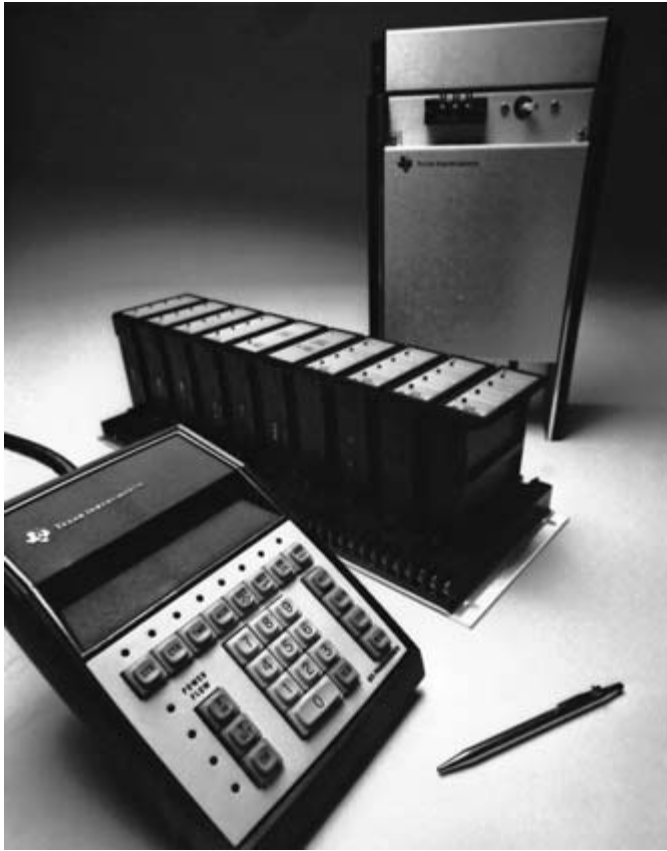
Fig. 2.14 A programmable logic control system ( Texas Instruments Ltd ).
